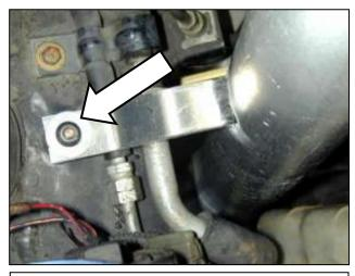
f. Install the washer and the lock nut onto the rubber mount.
