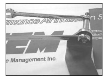
c. Install the factory mounting stud on the supplied engine mount bracket using the supplied nylock nut and washer.
