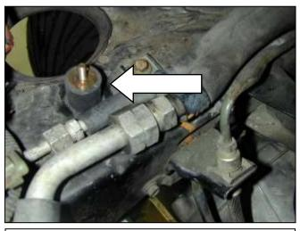
c. Install the rubber mount into the frame rail.
