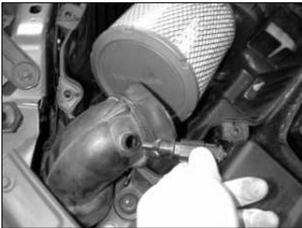
b. Remove the Inlet Air Temperature (IAT) sensor. The metal band will need to be pried off with a flat-head screwdriver. Use care to avoid damaging the IAT sensor.
