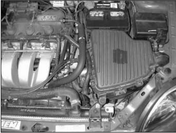
Factory air box system installed
