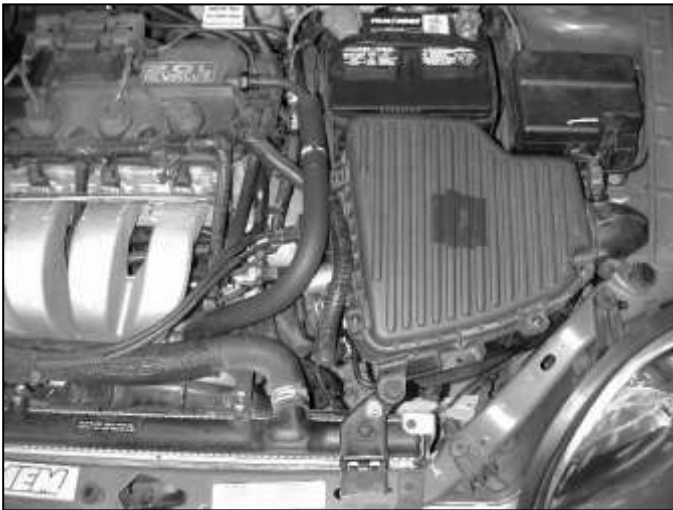
Factory airbox system installed
