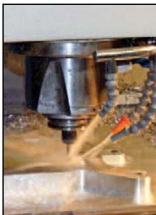
CNC Filter Mold Fabrication
