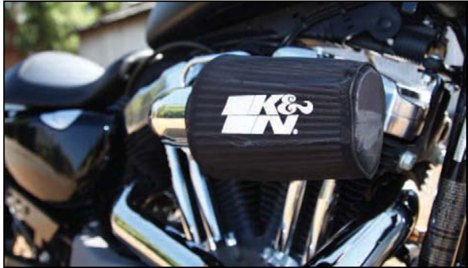
Aircharger® 63-1126P* and Precharger® RC-3680DK Installed
