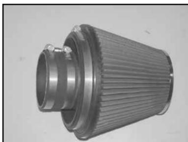
21. Install the silicone hose (08698) onto the K&N® air filter assembly and secure with the provided hose clamp.
