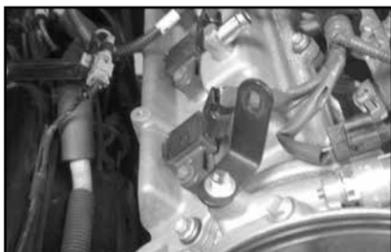
12. Install the small "L" bracket (070015) onto the threaded boss on the cam cover and secure provided bolt.
