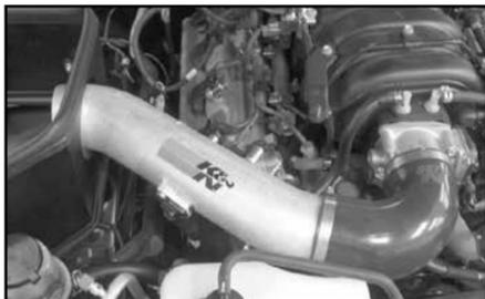
16. Install the K&N® intake tube into the throttle body and align with the mounting bracket installed in step #12. Secure with the provided hardware.
