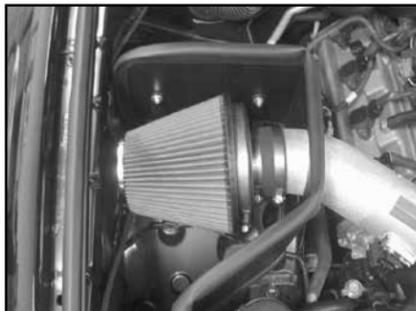
22. Install the air filter assembly onto the K&N® intake tube as shown and secure with the provided hose clamp.
