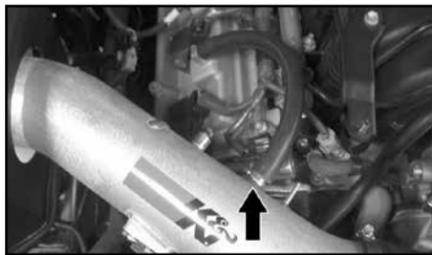
17. Remove the factory crank case vent hose from the valve cover and then install the supplied vent hose onto the valve cover and K&N® intake tube as shown.
