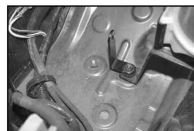
8. Remove the 12mm bolt that retains the power steering reserve to vehicle then mount the provided bracket (07158) onto the vehicle with the bolt that was removed.
