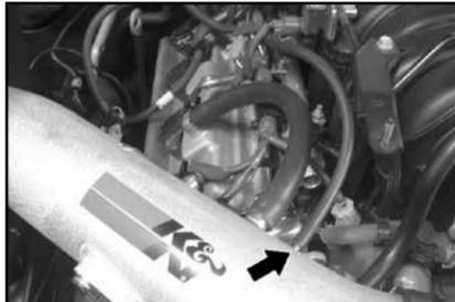
18. Connect the supplied fuel pressure regulator vent hose to the fuel pressure regulator and then onto the K&N® intake tube as shown.
