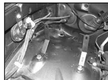
9. Mount the two provided brackets onto the vehicle with the provided hardware.
