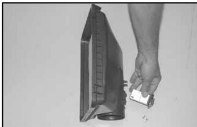
14. Remove the two screws that secure the mass air sensor to the air box lid, and then remove the mass air sensor as shown.
