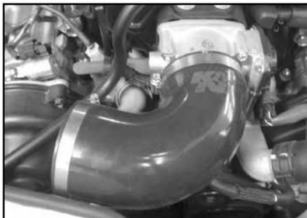
13. Install the silicone hose (084089) onto the throttle body and secure with the provided hose clamp.
