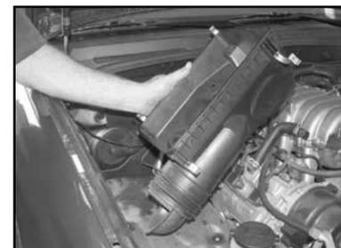
7. Remove the three bolts that retain the air box to vehicle, then remove the air box.
