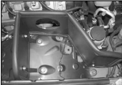
11. Install the heat shield onto the vehicle then secure to brackets with the provided hardware.
