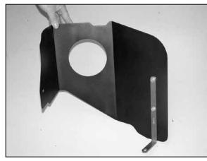
9. Install the "L" bracket (010060) onto the heat shield with the provided hardware as shown.
