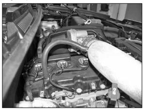
19. Install the provided crankcase vent hose onto the valve cover, then onto the  $K\&N^{\otimes}$  intake tube as shown.
