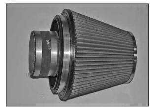
21. Install the silicone hose (08724) onto the air filter assembly as shown.
