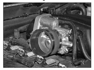
8. Install the silicone hose (08051) onto the throttle body and secure with the provided hose clamps as shown.
