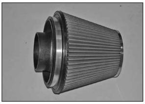
20. Install the filter adapter into the air filter and secure with the provided hose clamp. NOTE: Drycharger<sup>®</sup> air filter wrap; part # RF-1048DK is available to purchase separately.
