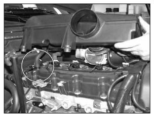
7. Remove the intake resonator from the engine as shown.
