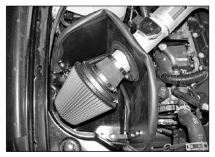
22. Install the air filter assembly onto the K&N<sup>®</sup> intake tube and secure with the provided hose clamp.
