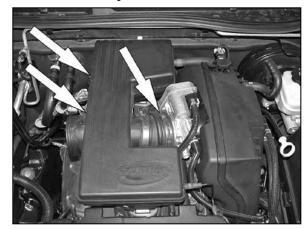
6. Loosen the two bolts that retain the intake resonator to the engine, and then loosen the hose clamp at the throttle body.
