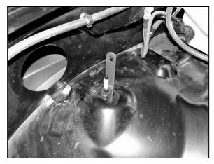
12. Install the "L" bracket (070602) onto the stock air box-mounting stud using the factory air box-retaining nut.
