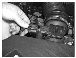
2. Depress the locking clip on the mass air sensor electrical connection, and then separate the mass air sensor electrical connection. 3. Loosen the hose clamp that retains the stock intake tube to the resonator, and then remove the tube from the resonator as shown.
