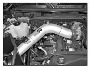
17. Install the K&N<sup>®</sup> intake tube into the silicone hose at the throttle body and through the heat shield, secure with the provided hose clamp.
