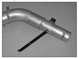
16. Install the small end of the tube-mounting bracket on the K&N<sup>®</sup> intake tube as shown. **NOTE: Do not completely tighten at this time.**
