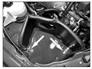
13. Install the heat shield into the vehicle using the hardware provided and the factory air box retaining nut.
