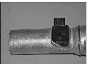
15. Install the mass air sensor into the K&N® intake
