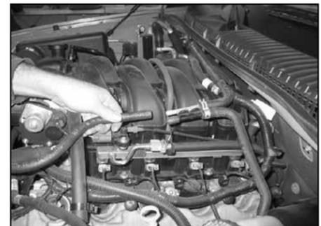
4. Disconnect the brake booster vent hose from the fitting as shown.
