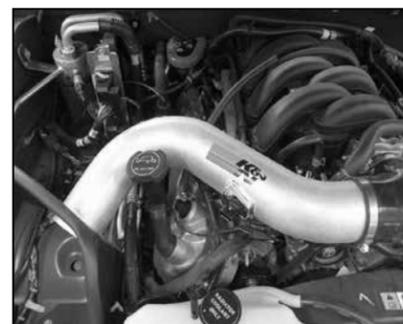
25. Install the K&N® intake tube into the silicone hose at the throttle body and align with the mounting bracket installed in step #22. Secure the intake tube with the hose clamp and supplied hardware.
