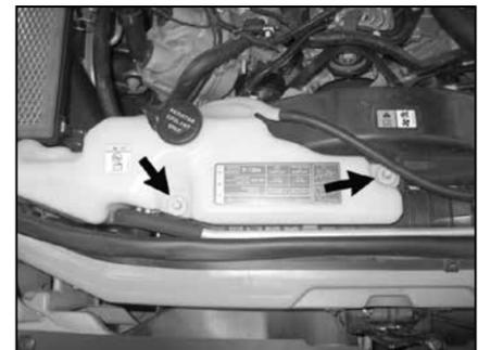
8. Loosen and remove the two bolts that secure the coolant recovery tank to the radiator.
