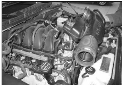
6. Remove the stock intake tube from the vehicle as shown.
