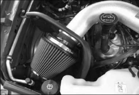
30. Install the air filter assembly onto the K&N® intake tube and secure with the provided hose clamp.
