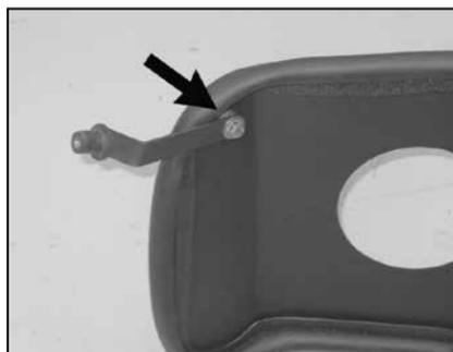
19. Attach the mounting bracket assembly to the heat shield with the provided hardware as shown.
