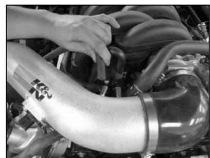
26. Install the supplied shorter crankcase vent hose onto the fitting on the valve cover and then onto the on the K&N® intake tube as shown.
