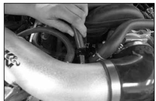
27. Install the supplied brake booster vent hose onto the factory fitting and then connect the other end to the fitting on the K&N® intake tube as shown.
