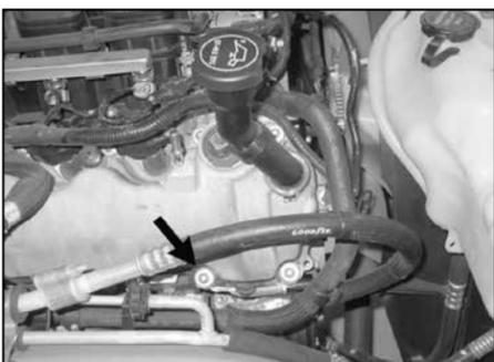
14. Remove the valve cover mounting bolt shown.
