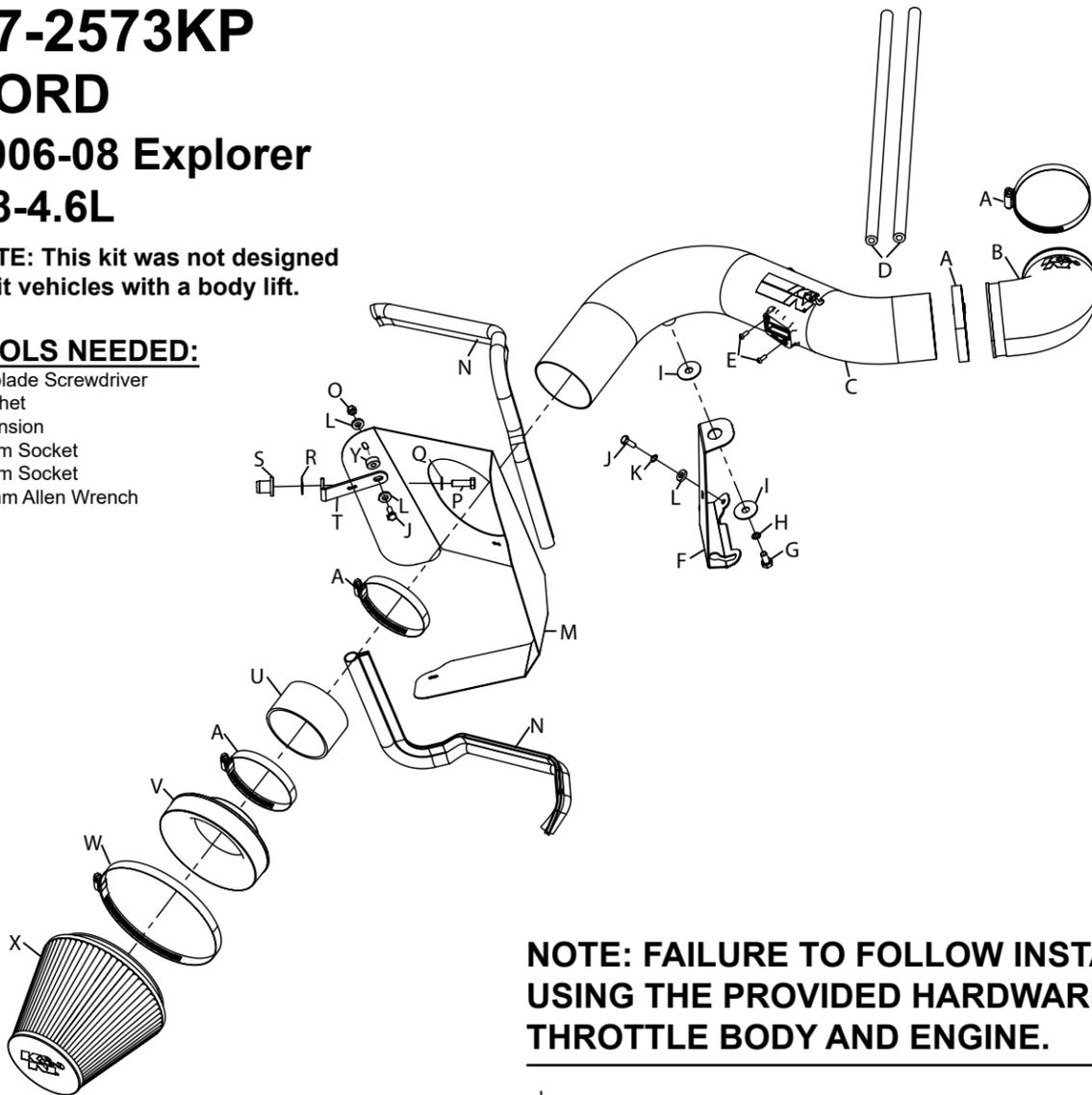
**NOTE: FAILURE TO FOLLOW INSTALLATION INSTRUCTIONS AND NOT USING THE PROVIDED HARDWARE MAY DAMAGE THE INTAKE TUBE, THROTTLE BODY AND ENGINE.**
