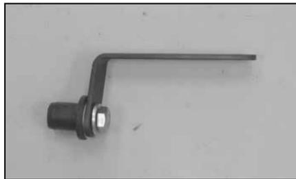
18. Attach the inserted nut to the mounting bracket with the hardware as shown.
