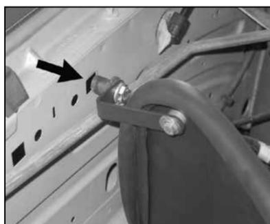
20. Install the heat shield assembly into the vehicle so that the inserted nut will fit into the hole in the inner fender panel.
