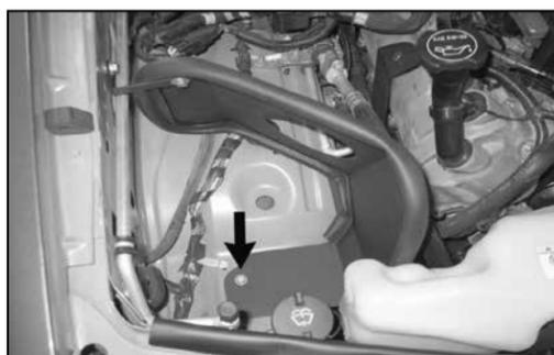
21. Secure the heat shield to the inner fender with the bolt removed in step #13 and the inserted nut and bolt.
