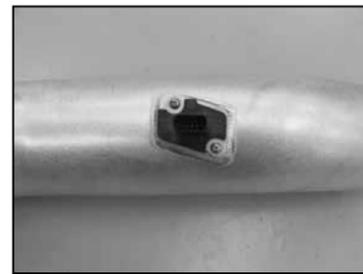
24. Install the mass air sensor assembly into the K&N® intake tube and secure with the provided hardware.
