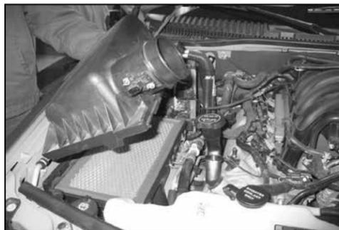
7. Unlatch the three airbox lid latches and then remove the lid from the vehicle.
