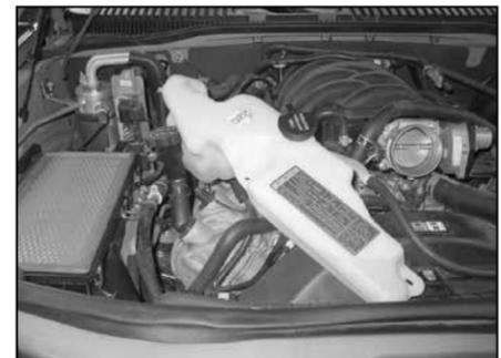
9. Lift and position the coolant recovery tank on the engine to gain access to the lower airbox.
