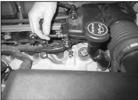
3. Disconnect the crankcase vent hose from the valve cover as shown.
