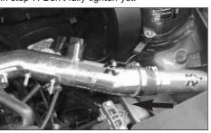
34. Slide the hose installed in step 32 over the intake tube as shown (direction indicated by the arrow) and secure both barrel clamps. Now adjust the tubes for best fit and clearance and tighten all securing hardware and hose clamps.
