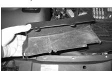
10. Remove the inner core support cover, which is secured by two screws.
