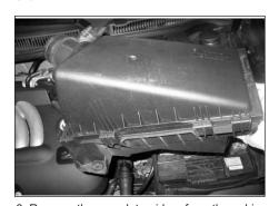
6. Remove the complete airbox from the vehicle as shown.
