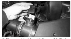
3. Disconnect the Mass Air Sensor (MAS) electrical connection as shown.
