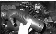
26. Undo the clamp and remove the complete intake hose from the vehicle as shown.
