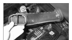
7. Remove the nut that secures the air inlet duct to the inner fender stud, then remove the inlet duct as shown. Attention: the nut will be
