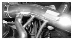
42. Refit the two vacuum hoses onto the intake tube as shown.
