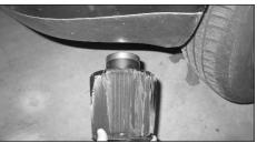
36. From underneath the vehicle install the filter onto the cold air tube using the hose clamp supplied.
