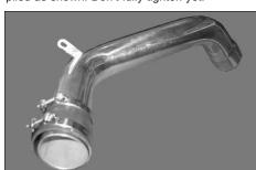
32. Install a silicone hose and the two barrel clamps onto the cold air extension tube as shown. Make sure to fit the hose over the non-swedged end of the tube & don't fully tighten yet!
