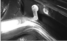
33. Fit the nylon spacer supplied over the stud on the inner fender. Now feed the swedged end of the cold air extension tube into the hole in the inner fender, then line up the bracket with the stud as shown and secure with the nut removed in step 7. Don't fully tighten yet!
