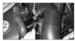
25. Remove the small vacuum hose underneath the crank case vent as shown.
