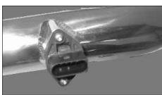
27. Mount the MAS onto the new intake tube using the two M5 bolts supplied.
