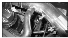
41. Fit the crank case vent hose onto the intake tube as shown.
