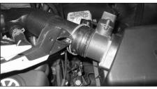
4. Carefully unclip the hose clamp from the MAS using a pair of pliers as shown.
