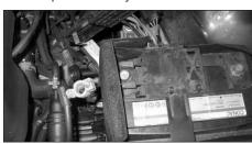
13. Disconnect the positive battery terminal as
