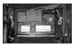
2. Remove the battery cover and disconnect the negative battery terminal.
