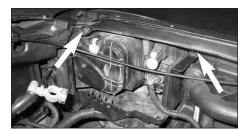
17. Remove the two indicated upper plastic rivets from the inner plastic headlight cover.
