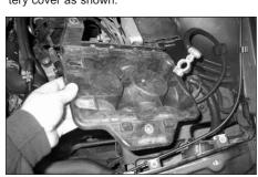
15. Remove the battery tray which is secured by four bolts.
