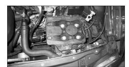
22. Reinstall the battery tray using the original four bolts
