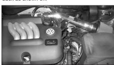
46. This K&N Typhoon intake kit has been designed to be used in two different configurations. In case of inclement weather, the cold air tube can be removed and the filter can be clamped onto the first intake tube located in the engine compartment as shown to avoid the possibility of ingesting water into the engine.
