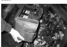
Remove the complete battery with the battery cover as shown.
