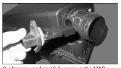
8. Unscrew and carefully remove the MAS from the airbox as shown.
