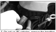
7. On set-up "B" vehicles, remove the breather hose from the side of the air box as shown.
