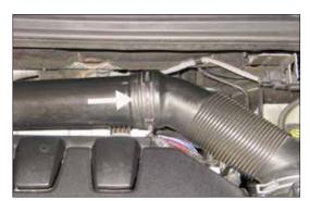
5. Release the spring clamp securing the factory intake hose to the factory intake tube and then unhook the intake hose.
