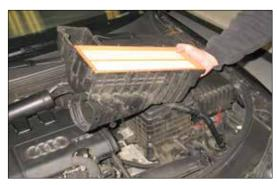
10. Lift the air box up to dislodge it from the mounting grommets and then remove it from the vehicle.
