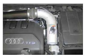
24. Install the K&N® secondary intake tube into the silicone hose at the factory intake tube and secure with the provided hose clamp.
