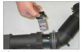
22. Remove the screws securing the mass air sensor and then remove the mass air sensor from the factory air box.
