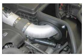
28. Install the provided silicone hump hose (08696) onto the K&N® primary intake tube and then install the primary intake tube into the heat shield. Secure the intake tube with the hose clamps and hardware provided to the mounting bracket and then connect the air injection hose to the factory air injection hose if equipped.
