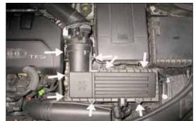
4. Loosen the eight screws securing the upper air box to the lower air box.
