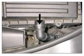
3. On vehicles equipped with an air injection system, release the air injection hose coupler from the upper air box half.
