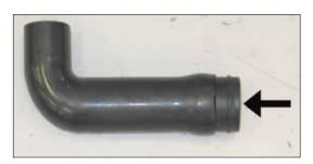
26. On vehicles equipped with an air injection system, install the provided coupler into the cut piece of air injection hose.
