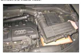
6. Remove the upper air box assembly from the vehicle as shown.
