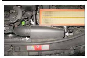
7. Release the three retaining clips securing fresh air intake lid and then remove the lid from the vehicle.
