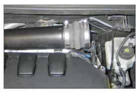
21. Install the provided silicone hump hose (08696) onto the factory intake tube and secure with the provided hose clamp.
