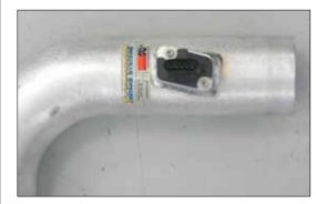
23. Install the mass air sensor into the K&N<sup>®</sup> secondary intake tube and secure with the provided hardware.
