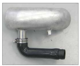
27. Install the air injection hose assembly onto the K&N® primary intake tube as shown and secure with the provided hose clamp. On vehicles not equipped with air injection, install the provided cap plug onto tube and secure with the provided hose clamp.
