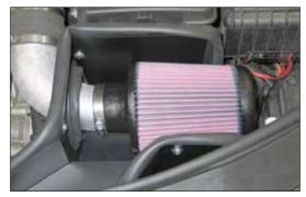
29. Install the K&N® air filter onto the primary intake tube, adjust the filter for adequate clearance and then tighten all of the hose clamps and tube mounting bracket.
