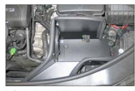
20. Set the heat shield into position on the air box mounting studs as shown and secure the mounting bracket with the provided hardware.
