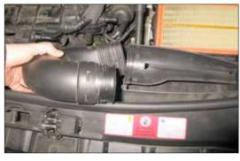
8. Disengage the fresh air intake duct from the lower air box and then remove the duct from the vehicle.
