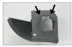
17. Install the 13" length of edge trim into the hole of the heat shield as shown.
