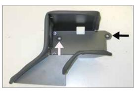
18. Install the two grommets into the base of the heat shield as shown.
