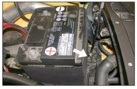
41. Reinstall the battery and the battery hold down block and secure as shown.
