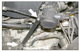
29. Secure the provided bracket to the mass air sensor using the provided hardware, then secure the other end to the battery tray using the stock air cleaner bolt as shown.
