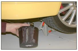
40. From underneath the vehicle install the filter onto the cold air tube and secure with the provided hose clamp.
