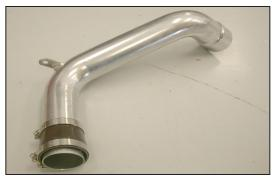
36. Install the silicone hose and hose clamps onto the K&N $^{\odot}$  cold air tube as shown.
