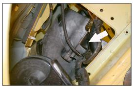
23. From underneath the vehicle remove the lower plastic rivet from the inner plastic headlight cover as shown.
