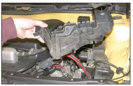
24. Remove the inner plastic headlight cover as shown.
