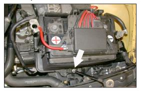
14. Remove the battery hold down block as shown.
