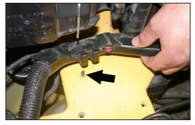
25. Remove the wire harness from the stud on the inner fender as shown.
