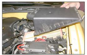
2. Depress the tabs on the side of the battery cover and remove as shown.
