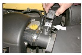
4. Disconnect the mass air sensor electrical connection as shown.
