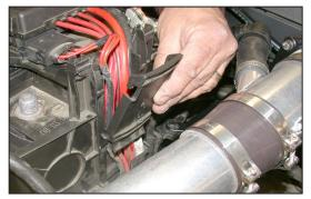
44. Slide the rear battery harness cover back onto the battery cover as shown.
