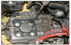
27. Reinstall the battery tray using the original four bolts as shown.
