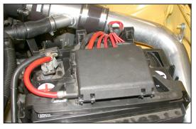
43. Reverse the removal process and slide the battery fuse/harness onto the battery cover as shown.
