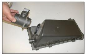
9. Remove the mass air sensor from the air cleaner cover as shown.
