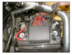
45. Reconnect the positive battery cable, and then the negative battery cable as shown.
