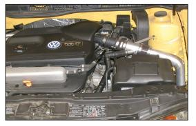
51. This K&N<sup>®</sup> high flow intake system has been designed to be used in two different configurations. In the case of inclement weather, the cold air tube can be removed and the air filter can be clamped onto the intake tube located in the engine compartment to avoid the possibility of ingesting water into the engine.
