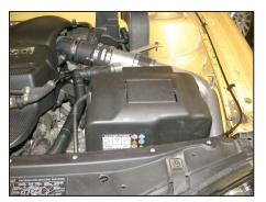
46. Reinstall the battery cover as shown.
