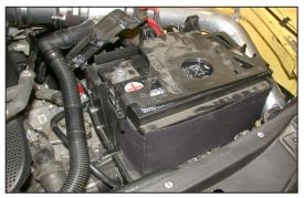
42. Reinstall the secondary battery cover as shown.
