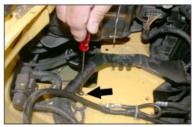
26. Using the provided plastic clamp secure the harness to the inner fender using the provided hardware as shown.
