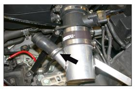
34. Slide the silicone hose onto the vent of the K&N<sup>®</sup> intake tube and secure with the provided hose clamp as shown.
