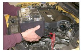
19. Remove the battery as shown.
