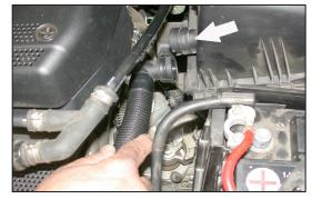
7. Disconnect the air pump vent hose as shown.
