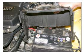
18. Remove the battery cover as shown.
