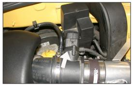
50. Reconnect the mass air sensor electrical connection as shown.
