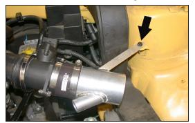
31. Slide the short K&N<sup>®</sup> intake tube into the silicone hose and secure the tube bracket to the original air cleaner mounting hole using one of the air cleaner bolts removed earlier.
