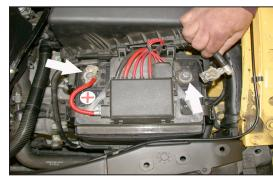
3. First disconnect the negative battery cable, then disconnect the positive battery cable as shown.
