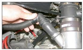
35. Reconnect the hard line to the plastic fitting as shown.
