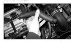
5. Unclip and remove the breather hose from the vehicle.
