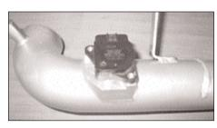
16. Carefully install the MAS into the intake tube using the two M4 Allen head bolts supplied.
