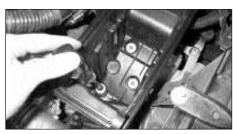
9. Remove the filter and undo the three bolts at the bottom of the air box base.
