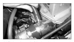
21 Fit the other end of the breather hose onto the intake tube.
