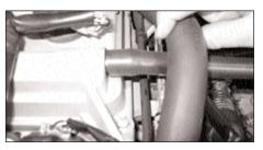
20. Fit the provided silicone breather hose to the breather tube on the valve cover.
