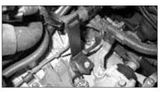
13. Mount the L-bracket to the air box mounting point using the M6 Allen head bolt and wave washer supplied.
