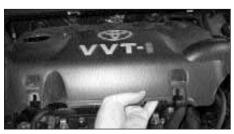
4. Undo the four bolts and remove the engine cover from the vehicle.
