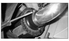
24. From underneath the car, slide the filter onto the intake tube & tighten the hose clamp.
