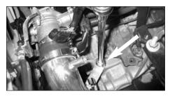
18. Secure the bracket to the threaded hole in the transmission housing using the M10 bolt and wave washer supplied.
