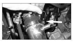
19. Tighten the hose clamp to secure the tube into the silicone hose.
