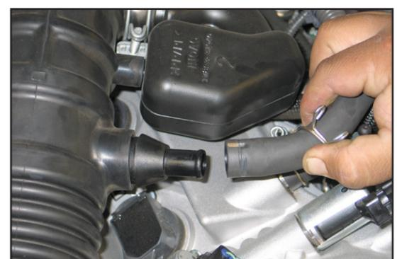
9. Unhook the crank case vent hose from the fitting in the stock intake tube.
