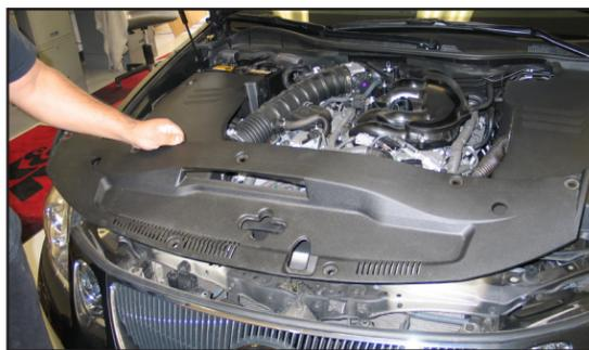
4. Remove the seven fasteners, then remove the cover from the core support.
