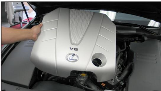
2. Pull firmly up on the engine cover and remove the cover from the engine as shown.
