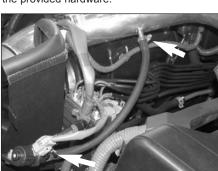
28. Connect the provided silicone hose to the evap solenoid, then, connect the other end to the vent on the K&N® intake tube with the provided hose clamps as shown.
