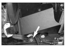
18. On 2002-2005 models slide the ABS pump bracket back to its original position and secure using the stock hardware as shown.
