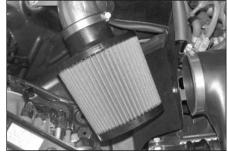
30. Install the K&N $^{\!0}$  air filter and secure with the provided hose clamp as shown.
