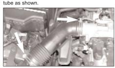
6. Loosen the 2 hose clamps that secure the intake tube to the air box and the throttle body.
