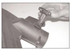
22. Remove the mass air from the factory air box as shown.
