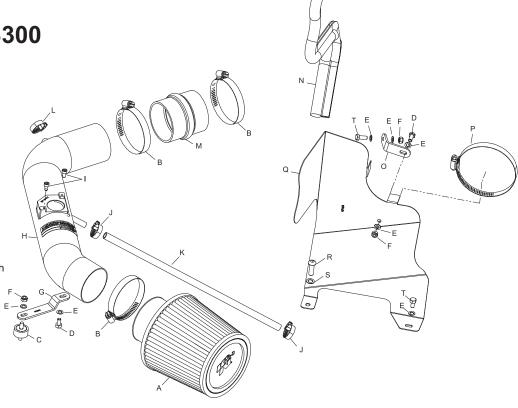
NOTE: FAILURE TO FOLLOW INSTALLATION INSTRUCTIONS AND NOT USING THE PROVIDED HARDWARE MAY DAMAGE THE INTAKE TUBE, THROTTLE BODY AND ENGINE.
