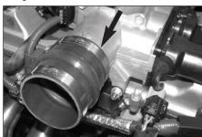
19. Using the provided hose clamps secure the provided silicone hump hose to the throttle body as shown.
