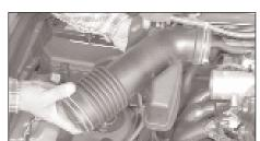
7. Remove the intake tube as shown.
