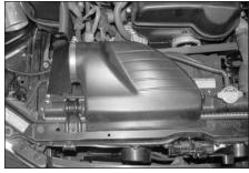
29. Using the stock hex bolt, secure the air inlet duct to the stock location on the radiator core support, then, use the provided hose clamp to secure the duct to the heat shield as shown.
