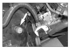
20. Install the rubber mounted stud to the original air cleaner mount as shown.
