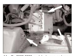
14a. On 2002-2005 models, loosen and remove the 2 bolts and one nut that retains the ABS pump to the vehicle. **NOTE: The nut is located on the back side of the ABS pump.**
