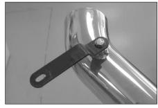
21. Secure the provided bracket to the K&N  $^{\! \otimes}$  intake tube using the provided hardware as shown.
