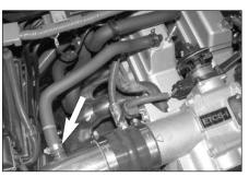
26. Remove the stock spring clamp and secure the crank case vent hose to the vent on the K&N® intake tube using the provided hose clamp as shown.
