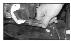
16. On 2002-2005 models slide the ABS pump inward to gain clearance for installation of the heat shield
