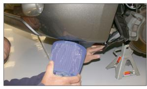
32. From underneath the vehicle pull the inner fender valance down, then, slide the air filter onto the cold air tube and secure with the provided hose clamp.
