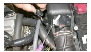
4. Using a flat blade screwdriver unclip the wire harness as shown.
