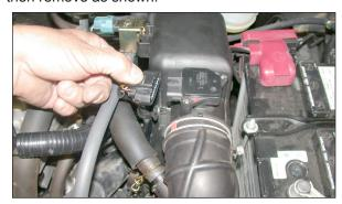
3. Disconnect the mass air sensor electrical connection as shown.
