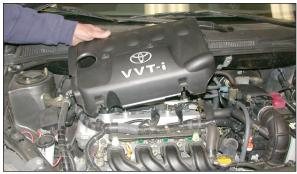
2. Remove the 4 bolt securing the engine cover, then remove as shown.
