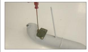
25. Install the stock mass air sensor into the K&N® cold air tube and secure with the provided hardware as shown.
