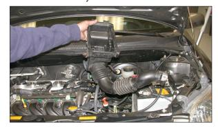
14. Pull upwards to remove the lower air cleaner assembly as shown.
