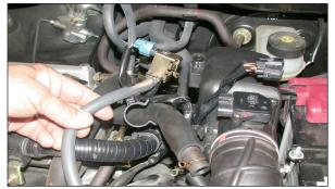
8. Unclip the vacuum hose from the crank case vent hose as shown.
