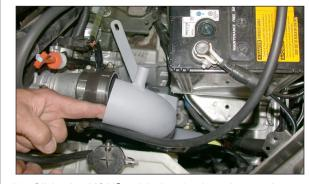
26. Slide the K&N $^{\!0}$  cold air tube into the engine compartment as shown.
