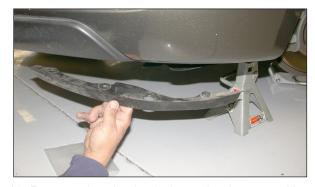
19. Remove the plastic air damn that is secured by three bolts, then remmove as shown.
