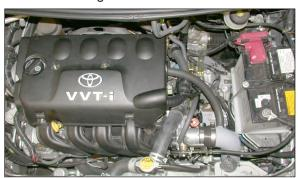
36. Reconnect the vehicle's negative battery cable. Double check to make sure everything is tight and properly positioned before starting the vehicle. WARNING: Please follow these installation instructions carefully. The K&N® high flow intake system is a performance product that can be used safely during mild weather conditions. During harsh and inclement weather conditions, you must return your vehicle to stock
