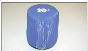
31. Install the Drycharger® onto the K&N® air filter as shown.
