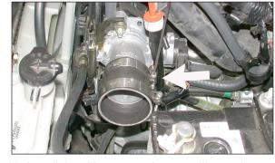
23. Install the silicone step hose and hose clamps onto the throttle body and tighten as shown.
