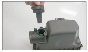
24. Remove the mass air sensor from the upper air cleaner assembly as shown.
