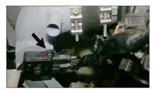
28. Reconnect the mass air sensor electrical connection using the provided hardware as shown.
