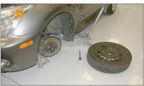
18. Raise the vehicle up and support it with jack stands, then, remove the front driver side tire as shown.
