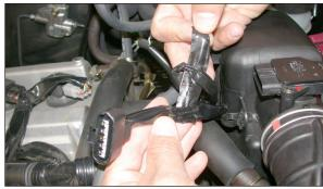
5. Remove the tape that binds the mass air sensor wire harness to the vacuum switching valve wire harness as shown.
