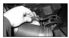
5. Remove the small breather hose from the intake tube as shown.
