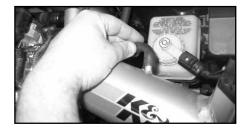
22. Fit the small breather onto the intake tube.
