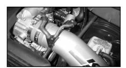
16. Fit the new intake tube into the silicone hose using the #48 hose clamp supplied. (do not fully tighten at this moment.)
