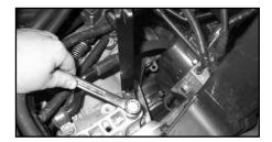
20. Now firmly tighten the gear box mounting bolt and the M6 bolt on the intake tube.
