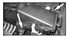
4. Remove the two bolts securing the air box and remove the complete airbox.
