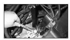
10. Mount the "Z" bracket onto the gear box mount using its original bolt. (do not fully tighten yet!)
