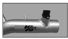
14. Mount the MAS onto the new intake tube using the two M5 bolts supplied. **NOTE**: Before installing , inspect the inside of the tube for any debris, then clean the inside out with water and a towel.
