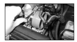
15. Install the silicone hose onto the throttle body using the #48 hose clamp supplied.
