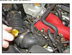
4. Loosen the hose clamp as shown.
