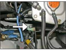
26. Use the remaining stock air cleaner hex bolt to secure the heat shield as shown.
