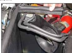
28. Install the remaining trim seal onto the heat shield and trim to fit as shown.
