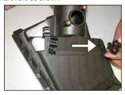
19. Remove one of the hose clips from the stock airbox assembly as shown.
