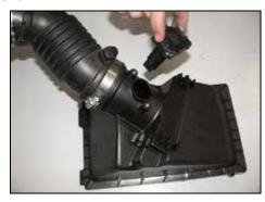
7. Remove the mass air sensor from the upper air cleaner assembly as shown.
