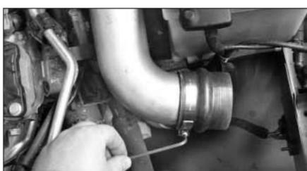
23. Secure the silicone hump hose onto the A-tube using a #40 hose clamp supplied.
