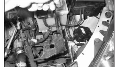
13. Remove the complete airbox mounting bracket by pulling it upwards.
