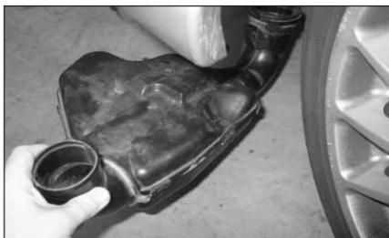
10. Remove the resonator box from the vehicle as shown by pulling it backwards.
