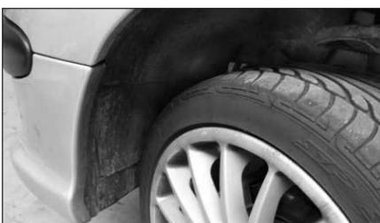
30. Re-install the wheel arch liner to the vehicle using the original hardware.
