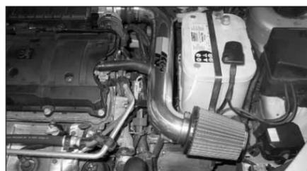
33. This Typhoon kit has been designed to be used in two different configurations. In case of inclement weather, the filter element can be clamped directly onto the A-tube to prevent water ingestion.
