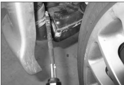
9. Unclip the indicated hose clamp securing the intake snorkel to the resonator box.
