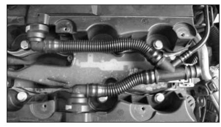
16. Re-install the breather assembly onto engine.
