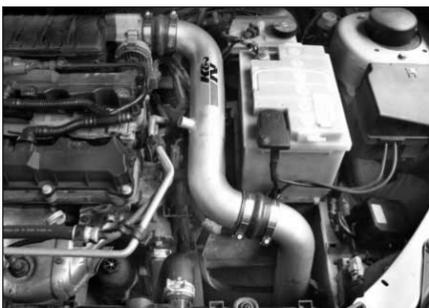
26. Align the A- and B-tube for best fit and clearance; now firmly tighten all hose clamps and hardware.
