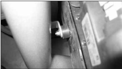
25. Align the welded-on bracket on the B-tube with the rubber vibration stud and secure using an M6 nylock nut and washer. Do not fully tighten yet!
