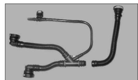
15. Carefully remove the breather pipe from the breather assembly as shown; it may be necessary to gently warm the pipe to do so.
