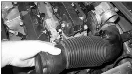
4. Unclip and remove the intake hose from between the throttle body and air box.
