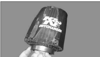
27. Fit the Drycharger onto the filter as shown.
