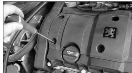
31. Re-install the engine cover to the engine, using the original hardware.
