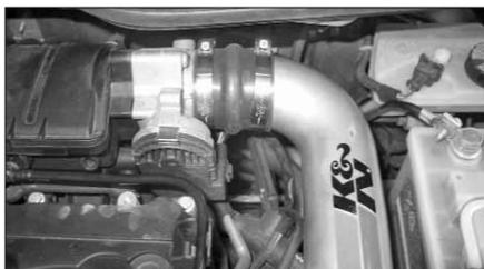
21. Feed the A-tube into the silicone hump hose and secure it with a #40 hose clamp supplied. Do not fully tighten yet!
