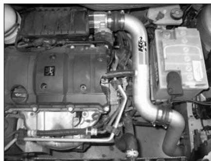
32. Reconnect the negative battery terminal. Installation is now complete.
