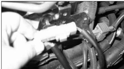
18. Remove the indicated (yellow) electronic connector from the bracket and insert it into another hole in the bracket as shown.
