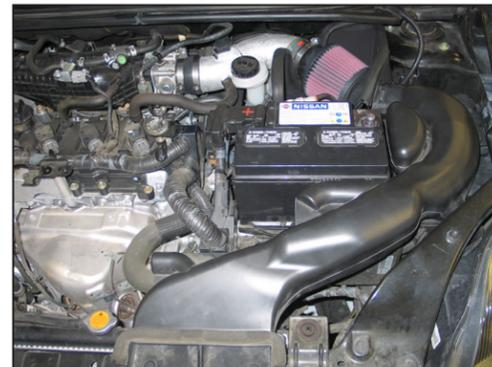
24. Reinstall the fresh air supply duct and secure with the factory plastic retaining clips.
