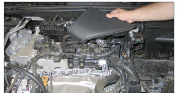
8. Remove the resonator mounting bolt and loosen the hose clamp which secures the resonator to the intake tube. Remove the intake resonator from the vehicle.
