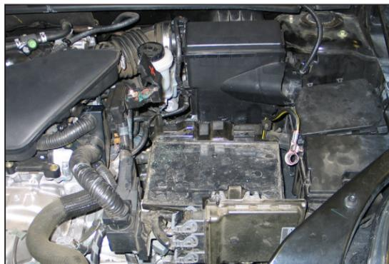
5. Remove the battery from the vehicle.
