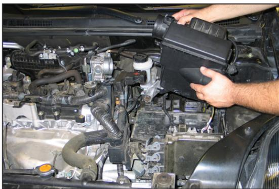
12. Remove the airbox from the vehicle.
