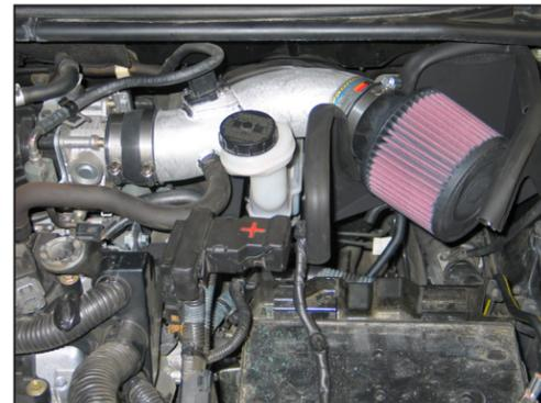
22. Install the K&N® air filter onto the K&N® intake tube and secure with the provided hose clamp.
