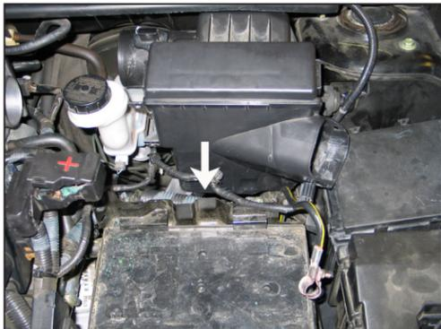
11. Remove the airbox mounting bolt located below the wiring harness, between the battery tray and airbox.
