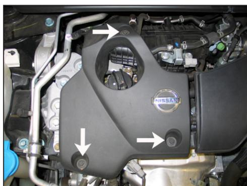
6. Remove the three bolts which secure the engine cover and then remove the engine cover.
