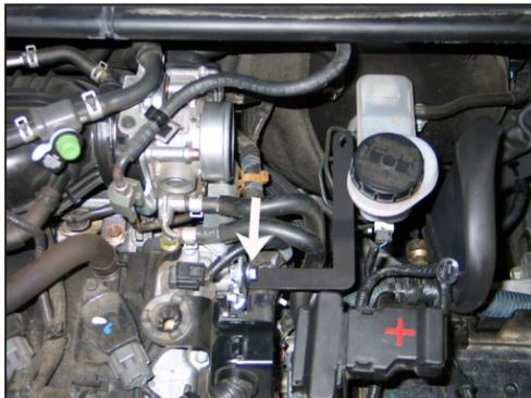
18. Install the intake tube mounting bracket onto the engine lifting bracket and secure with the provided hardware.
