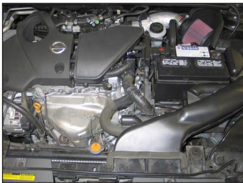
27. Reinstall the engine cover and secure with the factory bolts.
