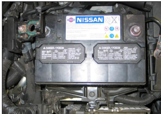
4. Disconnect the positive battery cable, then loosen the bolt and remove the battery hold down bracket.
