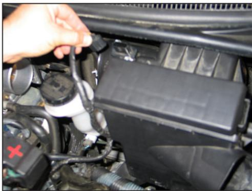
10. Disconnect the mass air sensor electrical connection and then release the harness from the airbox.
