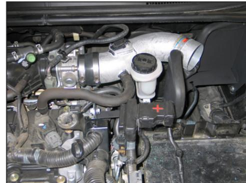
21. Install the crankcase vent hose onto the K&N® intake tube and secure with the factory hose clamp.
