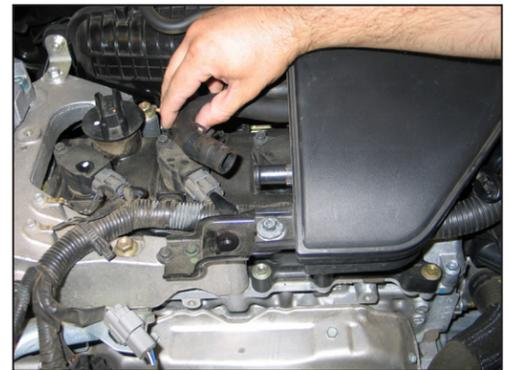
7. Release the spring clamp which secures the crankcase vent hose to the intake plenum and then disconnect the crankcase vent hose.
