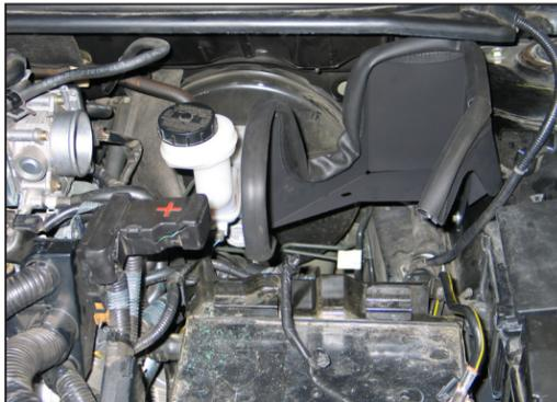
16. Secure the heat shield to the inner fender using the provided hardware.
