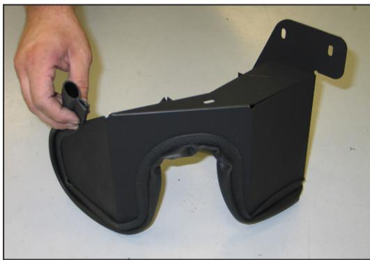
15. Install the provided edge trim onto the heat shield.
