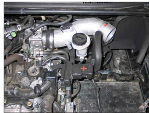
20. Install the K&N® intake tube into the silicone hose on the throttle body and align with the mounting bracket installed in step #19. Secure with the provided hardware and hose clamp.
