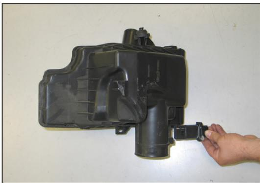
13. Remove the mass air sensor from the factory airbox.
