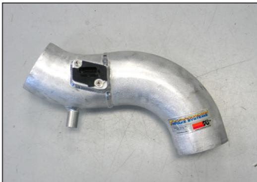
14. Install the mass air sensor into the K&N® intake tube and secure with the provided hardware.
