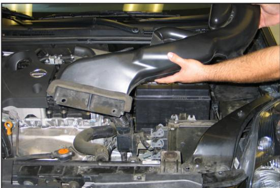
3. Remove the fresh air supply duct from the vehicle.
