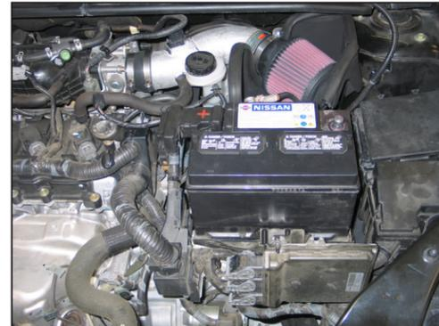
23. Reinstall and secure the battery, reconnect the positive battery cable.
