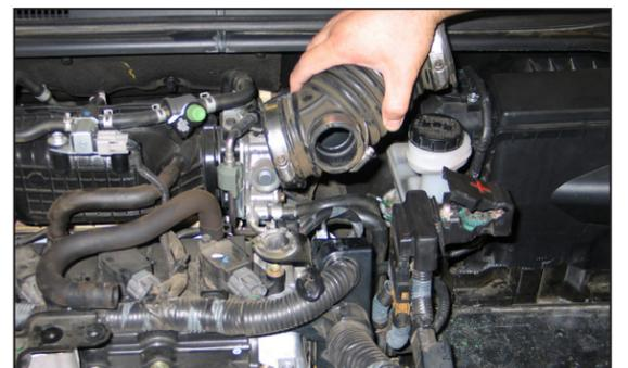
9. Loosen the hose clamps which secure the intake tube and then remove the intake tube from the vehicle.
