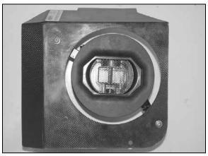
35. Center the heat shield around the mass air adapter, then secure it using th provided hardware as shown.
