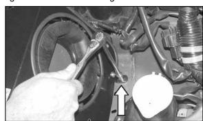
42. Secure the angle bracket to the inner fender using the provided hardware as shown.
