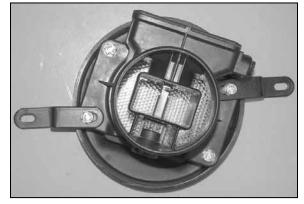
34. Assemble the mass air adapter, "Z" brackets, and the stock mass air gasket onto the stock mass air sensor as shown.
