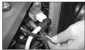
18. Remove the lower bolt that secures the air bag sensor to the radiator core support as shown. (Except UK)
