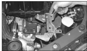
9. Lift up the air cleaner support bracket and unclip the wire harnesses, then, remove the bracket as
