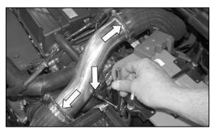
4. Loosen the three hose clamps on the intercooler tube as shown.
