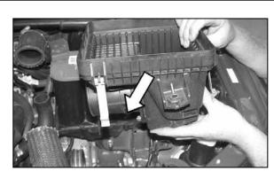
7. Remove the two bolts on the lower air cleaner assembly, then, lift up the lower assembly to unclip the mass air sensor electrical connection. Unclip the mass air sensor wire harness from the bottom the lower air cleaner assembly, then, remove the lower air cleaner assembly as shown.
