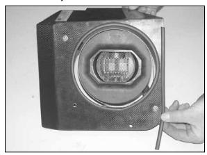
38. Apply the remaining piece of trim seal to the edge of the heat shield as shown.
