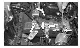
8. Remove the four bolts that secure the air cleaner support bracket to the inner fender as shown.
