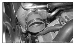
24. Install the silicone step hose and hose clamps onto the turbo inlet and tighten as shown.
