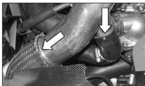
44. Slide the intercooler tube into the intercooler hose and reconnect the bypass valve to the vent on the intercooler tube as shown.
