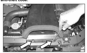
2. Depress the center pins on the plastic rivets that secure the air inlet duct to the radiator core support as shown.
