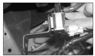
21. Using the hex nut from step 10 secure the solenoid valve to the provided "Z" bracket as shown
