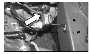
23. Install the provided silicone hose onto the solenoid valve as shown.
