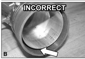
26. Install the provided silicon step hose onto the K&N® intake tube using the provided hose clamps as shown.
