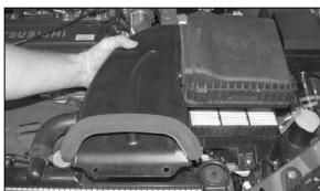
3. Unclip the upper air cleaner assembly and remove the complete assembly as shown.
