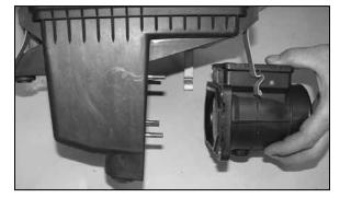
33. Remove the four hex bolts to remove the mass air sensor from the lower air cleaner assembly as shown.
