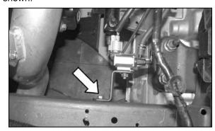
22. Secure the solenoid valve assembly to the inner fender using the provided hardware as shown.
