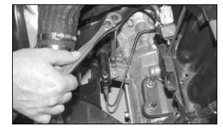
17. Remove the slave cylinder bolt as shown.
