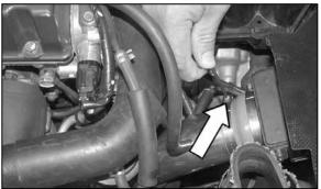
43. Tighten the hose clamp on the K&N $^{\! \rm 8}$  intake tube as shown.
