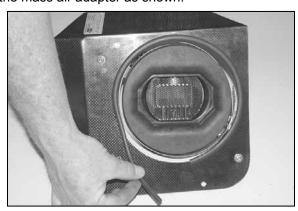
37. Install the provided edge trim onto the heat shield assembly and trim to fit as shown.
