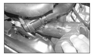
27. Slide the K&N® intake tube assembly into the silicone hose on the turbo as shown.
