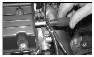
12. Disconnect the crank case vent hose from the cam cover as shown.
