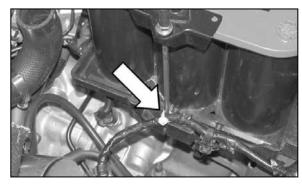
40. Using the provided zip tie secure the mass air sensor wire harness to the battery hold down bolt as shown.
