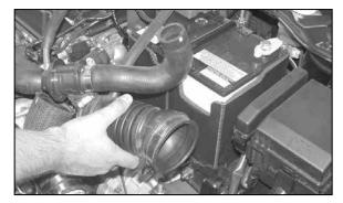
15. Loosen the hose clamp at the turbo inlet and remove the intake tube assembly as shown.
