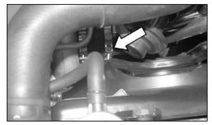
29. Tighten the hose clamp on the silicone hose on the turbo/intake tube as shown.
