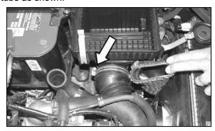
6. Loosen the hose clamp at the mass air sensor as shown
