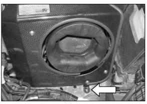
41. Slide the heat shield assembly onto the K&N® intake tube and line up the angle bracket with the original air cleaner mounting hole as shown.
