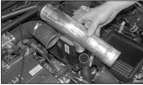
5. Pull firmly on the hoses to remove the intercooler tube as shown.
