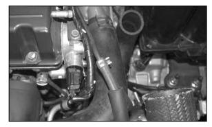
30. Reconnect the bypass valve vent hose to the hardline as shown.
