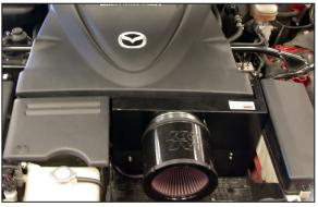
39. Install the engine cover as shown.
