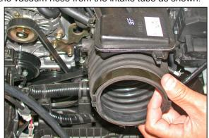
15. Remove the intake hose as shown.
