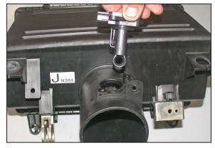
17. Remove the mass air sensor from the air cleaner housing as shown.
