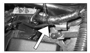
33. EU and UK SP-vehicles with the dummy electrical connection described in step 4, secure the excess electrical connector away using the zip tie provided as shown.
