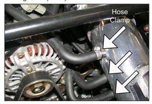
35. Connect the three vent lines to the K&N $^{\rm @}$  intake tube and secure with the provided hose clamps.
