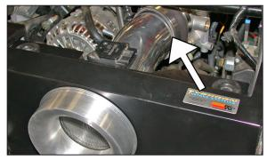
29. Install the heat shield into the vehicle and slide the intake tube into the silicone hose as shown.
