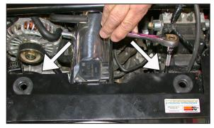
30. Secure the heat shield to the stock air cleaner mounts using the stock bolts as shown.
