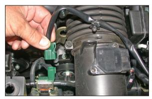
4. On manual transmission vehicle, (automatic transmission vehicles, go to step 7.) disconnect the vacuum switch electrical connection and unclip the wire from the mass air sensor housing as shown.
