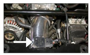
37. Reconnect the mass air sensor electrical connection as shown.
