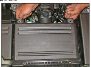
9. Lift up on the back of the air cleaner to release the airbox assembly from the stock grommets.
