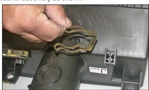
19. On manual transmission vehicles (automatic transmission vehicles go to step 20) remove the vacuum canister clip from the air cleaner assembly.
