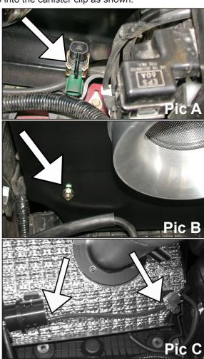
32. Manual transmission vehicles install the vacuum switching valve onto the back side of the heat shield (Pic A) and secure using the stock nut (Pic B) as shown.
