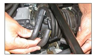
7. Disconnect the three hoses from the stock intake tube as shown.
