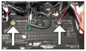
16. Remove the two lower bolts that secure the airbox assembly support brackets as shown.
