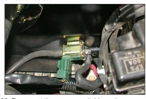
38. Reconnect the vacuum switching valve electrical connection as shown.
