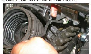
14. Loosen the hose clamp and pull the intake tube off of the throttle body, rotate the tube and unclip the vacuum hose from the intake tube as shown.
