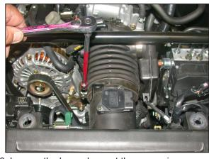
8. Loosen the hose clamp at the mass air sensor as shown.
