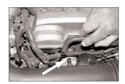
5. Disconnect the crankcase vent hose from the stock intake tube as shown.
