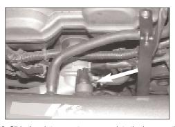
22. Slide the air temperature sensor into the bung on the  $K\&N^{\circledcirc}$  intake tube as shown.
