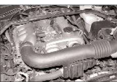
6. Loosen the hose clamps at the throttle body and at the mass air sensor, then remove the stock intake tube as shown.
