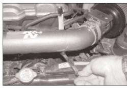
20. Tighten the hex bolt on the K&N® intake tube as shown.
