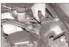
7. Loosen and remove the bolt that secures the air inlet duct to the inner fender, then remove the air inlet duct as shown.
