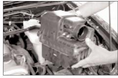
Pull upwards to remove the air cleaner assembly as shown.
