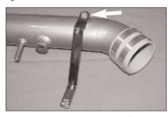
15. Install the "Z" bracket onto the K&N $^{\! \otimes}$  intake tube using the provided hardware as shown.
