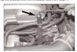
17. Using the provided hex bolt secure the bracket to the cam
