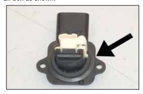
15a. Remove the o-rings and install the provided gaskets onto the mass air sensors as shown.
