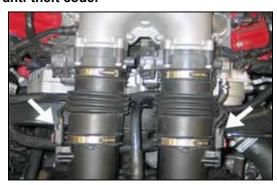
2. Release the locking tabs and then disconnect the two mass air sensor electrical connections.
