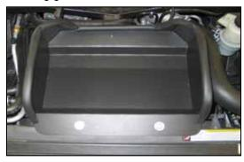
10. Install the heat shield onto the air box mounting location and secure with the provided hardware.
