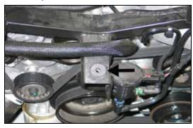
9. Install the provided nut insert into the air box mounting grommet hole as shown.
