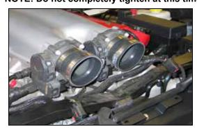
12. Install the silicone hoses (084091) onto the throttle bodies and secure with the provided hose clamps.
