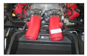
18. Install the right side K&N® intake tube into the silicone hose at the throttle body and then secure the tube to the mounting bracket with the provided hardware.
