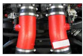
23. Reconnect the mass air sensor electrical connections.
