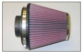
20. Install the filter adapters into the K&N® air filters and secure with the provided hose clamps.
