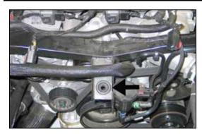
7. Remove the rubber mounting grommet shown.
