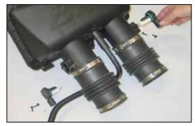
15. Remove the mass air sensors from the factory air box as shown.
