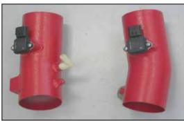
16. Install the mass air sensors into the K&N® intake tubes and secure with the provided hardware.
