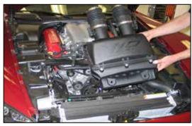
6. Dislodge the air box assembly from the mounting grommet and remove the air box from the vehicle. NOTE: K&N Engineering, Inc., recommends that customers do not discard factory air intake.
