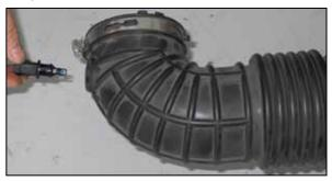
15. Remove the inlet air temperature sensor from the stock intake hose as shown. NOTE: Be very careful when handling the inlet air temperature sensor as it is very fragile. NOTE: The inlet air temperature sensor may be a different style than the one shown.
