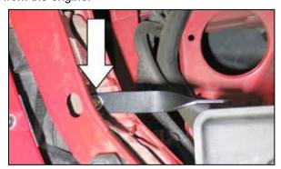
9. Install the twist bracket (070772) onto the core support using the provided hardware through the existing hole as shown.
