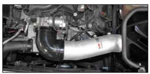
19. Install the K&N<sup>®</sup> intake tube into the silicone hose at the throttle body and align with the heat shield and mounting bracket. Secure the intake tube with the hose clamp and hardware provided.
