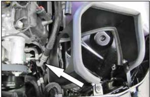
12a. Due to vehicle manufacturing tolerances, the A/C lines on some vehicles may need to repositioned slightly so that they do not contact the heat shield. To adjust, grab the A/C line on the aluminum section and carefully apply pressure in the desired direction until clearance is obtained.
