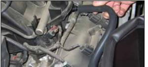
10. Install the "L" bracket (070066) onto the heat shield with the provided hardware through the non-slotted hole in the bracket.
