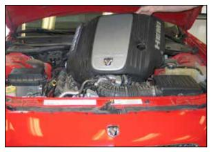
2. Lift up the engine cover to loosen it from the mounts, and then remove the cover from the vehicle.
