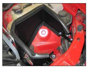
12. Install the heat shield assembly into the vehicle and secure to the bracket installed in step #9. Then secure the "L" bracket with the factory bolt removed in step #6 to the airbox mounting location.
