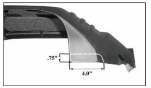
25a. It may be necessary on some vehicles to trim the engine cover as shown to clear the tube mounting bracket.
