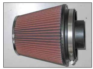
22. Install the provided air filter adapter into the K&N $^{\circ}$  air filter and secure with the provided hose clamp.
