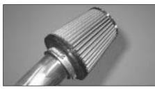
11. Clean the inside of the tube with water and a towel. Fit the filter to the tube using the hose clamp supplied.
