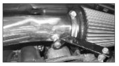
14. Fit the tube onto the "L" bracket using a washer, waved washer and M6 bolt supplied. Align the tube and tighten the hose clamp and M6 bolts.
