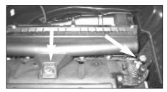
3. Unbolt and remove the two indicated bolts from the vehicle as shown.
