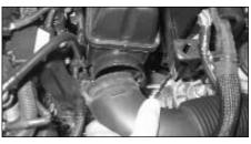
2. Remove the intake snorkel from the resonator box as shown.
