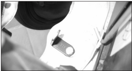
20. Fit the L-bracket to the inner fender using an M6 bolt and flat metal washer supplied. Make sure the short leg of the "L" sits on the fender. (don't fully tighten yet!)
