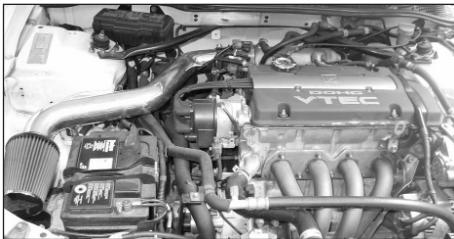
30. This Typhoon kit has been designed to be used in two different configurations. In case of inclement weather, the filter element can be clamped directly onto the A-tube to prevent water ingestion.
