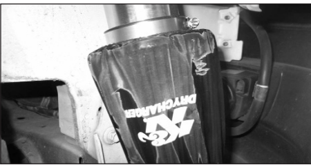
26. Mount the filter onto the B tube using the # 44 hose clamp supplied.
