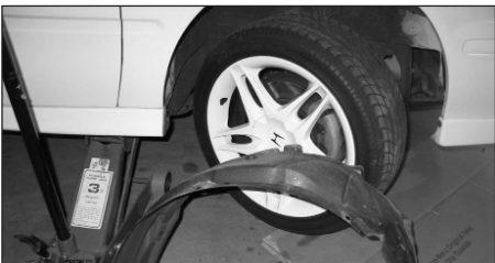
27. Re-install the wheel arch liner back onto the vehicle.
