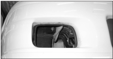
18. Remove the bolt that secures the resonator to the vehicle and remove the complete resonator box.
