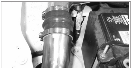
22. Feed the B-tube into the sleeve using a hose clamp supplied. (do not fully tighten at this moment.) NOTE: Before installing clean the inside of out with water and a towel!
