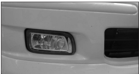
19. Re-install the fog light to the bumper. NOTE: Re-adjust the fog light as necessary to avoid blinding oncoming traffic!
