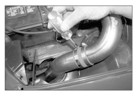
23. Line up the bracket on the cold air tube with the rubber mounted stud in the inner fender, then, secure the K&N® cold air tube to the silicone hump hose.
