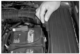
6. Release the clip on the cruise control cable.
