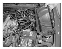
11. Loosen the two bolts that retain the lower air cleaner base, then, pull upwards to remove the air cleaner base as shown.
