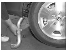
22. Install the K&N® cold air tube from underneath the vehicle as shown.
