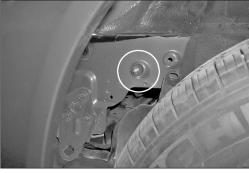
21. Install the rubber mounted stud into the threaded hole from the air intake resonator as shown.
