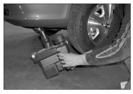
14. Loosen the two bolts that secure the air intake resonator to the inner body frame rail, then, remove the resonator from below the vehicle as shown.
