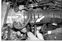
3. Using a pair of pliers, depress the stock hose clamp then remove the crank case vent tube from the stock intake tube as shown.
