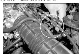
4. Disconnect the idle air bypass control thermal valve from the stock intake tube as shown.
