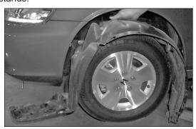
13. Using a flat blade screwdriver and a phillips screwdriver, remove the push clips and screws that retain the inner fender valance, then remove the valance as shown.
