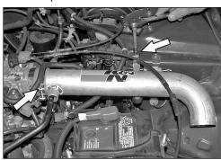
20. Slide the K&N® intake tube into the silicone hose on the throttle body, then, using the bolt removed in step 16, secure the "Z" bracket and the EVAP canister purge valve bracket to the stock mounting point as shown.
