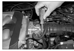
7. Using a phillips screwdriver, loosen the hose clamp at the throttle body as shown.
