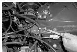
16. Remove the bolt that secures the EVAP canister purge valve bracket to the strut tower as shown.
