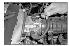
5. Disconnect the MAP sensor electrical connection as shown, then, move the connection out of the way for removal of the intake tube.
