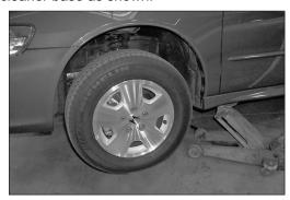
12. Using a floor jack, raise the driver front side of the vehicle up and support the vehicle with jack stands.
