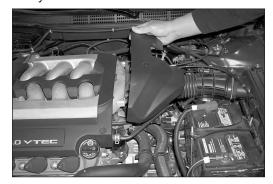
2. Remove the throttle body cover by turning the plastic pins 1/4 turn, then pull upwards to remove.
