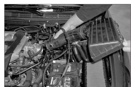
9. Lift up on the air cleaner lid, then, pull firmly on the stock intake tube to remove the upper air cleaner assembly as shown.
