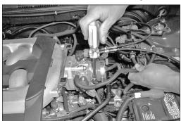
15. Install the provided silicone hose onto the throttle body, then, secure it with the provided hose clamps.
