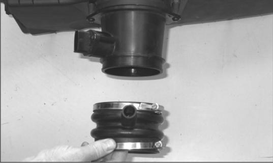
10. Loosen the hose clamp that secures the factory intake tube to the mass air sensor housing, then remove as shown.
