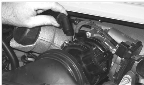
5. Remove the crank case vent line from the factory intake tube as shown.
