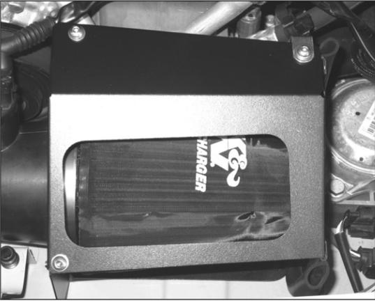
27. Install the heat shield top cover and mass air sensor harness clip (removed in step # 4) onto the heat shield with the provided hardware as shown.
