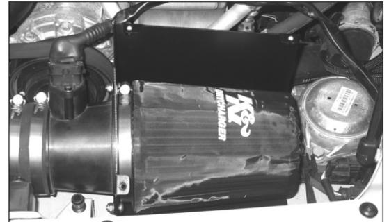
25. Install the K&N® air filter onto the K&N® intake tube and secure with the provided hose clamp as shown.
