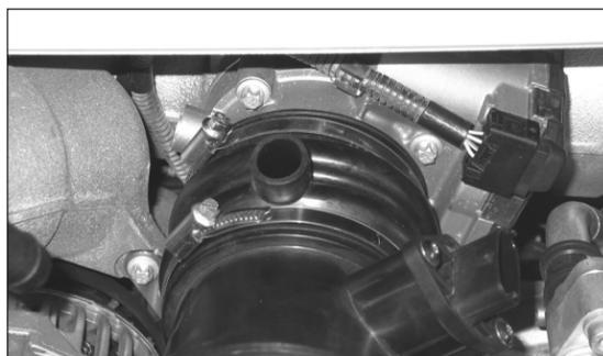
6. Loosen the hose clamp securing the factory intake tube to the throttle body. Pull the factory intake tube from the throttle body.
