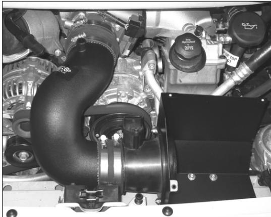
19. Install the K&N® intake tube onto the throttle body and mass air sensor housing. Secure with the provided hose clamps as shown.
