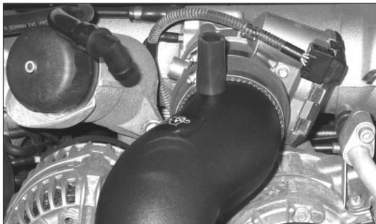
20. Install the provided silicone hose onto the K&N® intake tube as shown.
