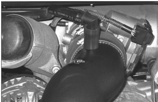
21. Re-connect the crank case vent line to the silicone hose installed in the previous step as shown.
