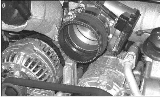
15. Install silicone hose (#08699) onto the throttle body and secure with the provided hose clamp as shown.
