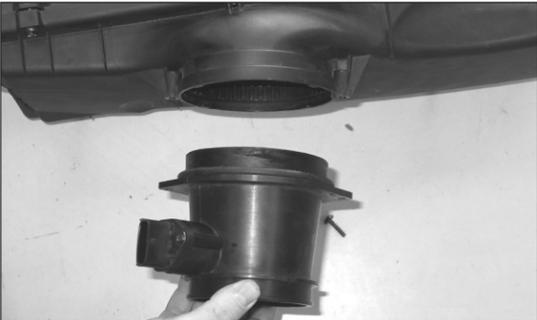
11. Remove the two torx screws that secure the mass air sensor to the factory air box. Remove the mass air sensor housing as shown.
