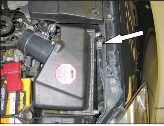
7. Remove the bolt that secures the airbox to the inner fender.
