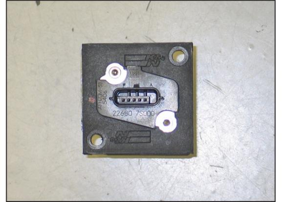
15. Install the mass air sensor into the K&N® mass air sensor adapter. Secure with the provided hardware.
