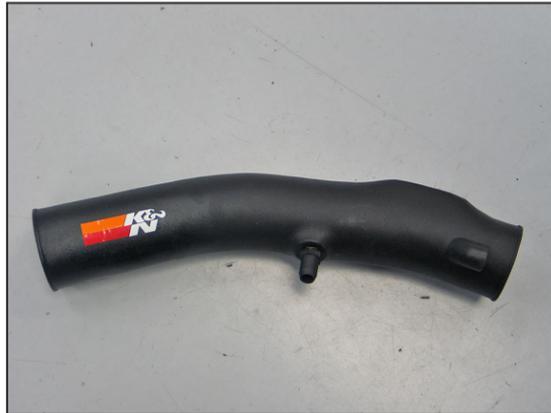
12. Install the 1/4" NPT fitting into the K&N® intake tube as shown.
