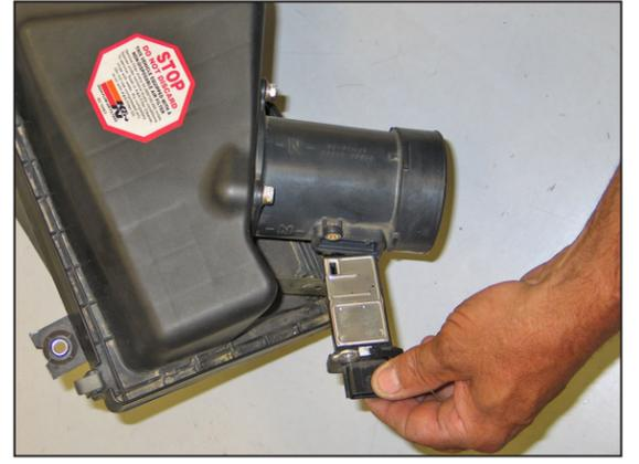
14. Remove the mass air sensor mounting screws. Then, remove the mass air sensor from the stock mass air sensor housing.
