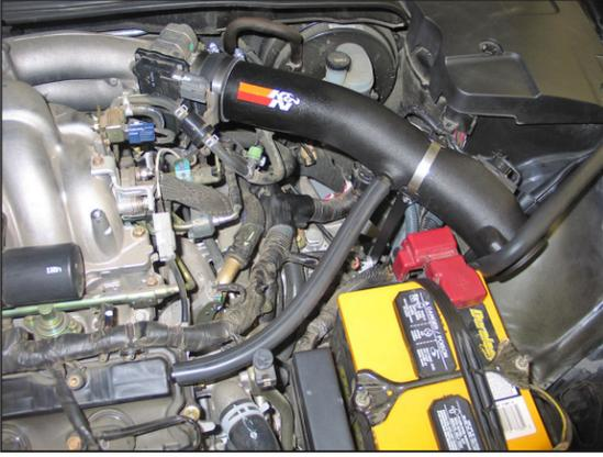
20. Install the provided crankcase vent hose onto the vent port on the valve cover. Connect the open end to the 1/4" NPT fitting installed into the K&N® intake tube.
