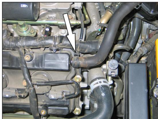
3. Release the spring clamp and disconnect the crankcase vent hose.
