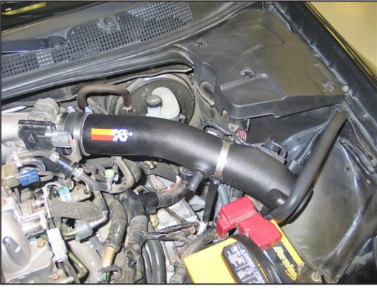
19. Install the K&N® intake tube assembly into the silicone hose at the throttle body and align with the saddle bracket installed in step #11. Secure the K&N® intake tube assembly with the provided hose clamps.
