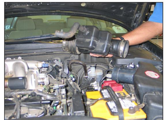
6. Remove the stock intake tube from the vehicle.
