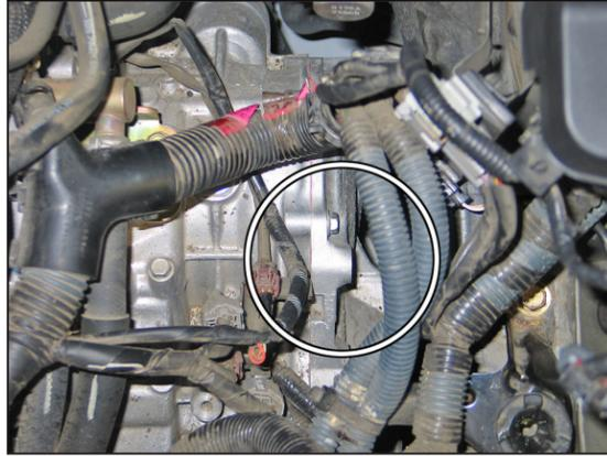
11. On 2004-2006 model vehicles, secure the tube mounting bracket assembly (06489) to the threaded boss on the transmission with the provided hardware.
