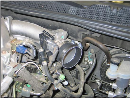
9. Install silicone hose (#08690) onto the throttle body and secure with the provided hose clamp.
