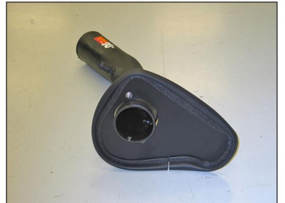
18. Secure the heat shield assembly to the K&N® intake tube with the provided hardware.
