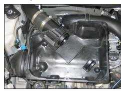
15. Install the air box onto the engine, connect the intake tube and secure with the provided hose clamp. Reinstall the retaining clips to secure the front of the air box. Reconnect the fresh air inlet tube to the air box.
