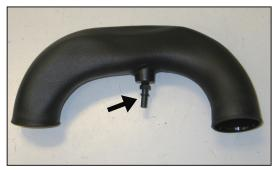
11. Install the provided crank case quick connect fitting into the K&N® intake tube as shown. **NOTE: Plastic NPT fittings are easy to cross**
