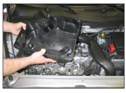
7. Remove the two clips securing the front of the air box to the engine and then remove the complete air box assembly from the vehicle.
