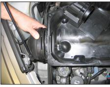
4. Disconnect the fresh air inlet duct from the air box as shown.
