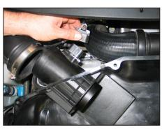
6. Disconnect the mass air sensor electrical connection.
