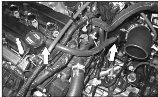
20. Install the provided crank case vent hose to the 1/4NPT X 1/2" on the K&N® intake tube and then attach the other end to the vent port on the valve cover as shown.
