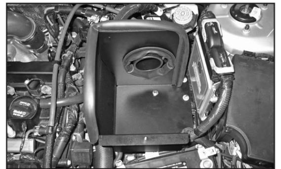
24. Install the heat shield onto the rubber mounted stud installed during step #13 and onto the ECU mounting studs. Then secure the heat shield with the factory ECU mounting bolts and hardware provided.
