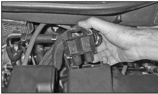
4. Release the clip which holds the vacuum switches to the upper air box and then unhook the vacuum switches from the air box.
