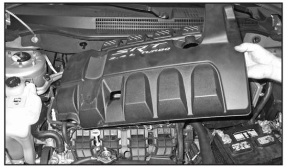
7. Lift up the engine cover to dislodge it from the mounting studs and then remove the engine cover from the vehicle.
