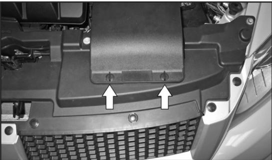
2. Unlock the two fresh air retaining clips by turning a ¼ turn counter clockwise.
