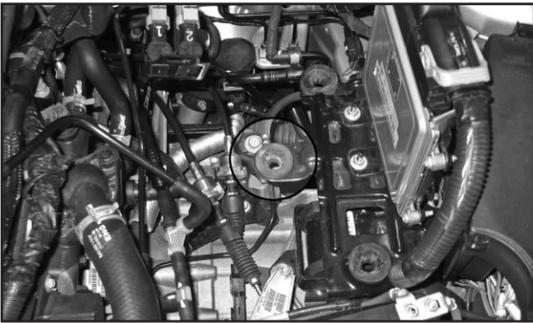
12. Remove the center air box mounting grommet shown.
