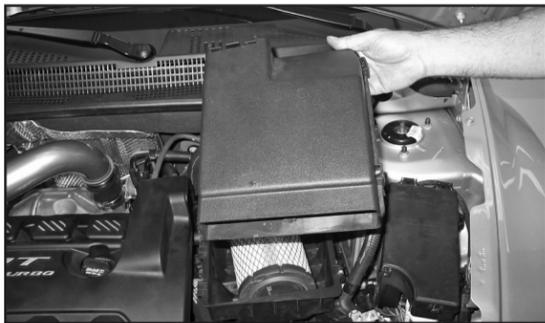
5. Unhook the upper air box retaining clips and then remove the upper air box as shown.
