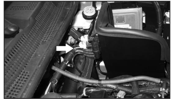
25. Secure the vacuum solenoids to the stud on the back of the heat shield using the provided hardware.
