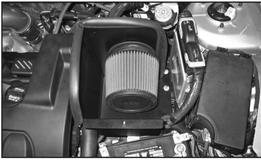
28. Install the K&N® air filter onto the intake tube and secure with the provided hose clamp.
