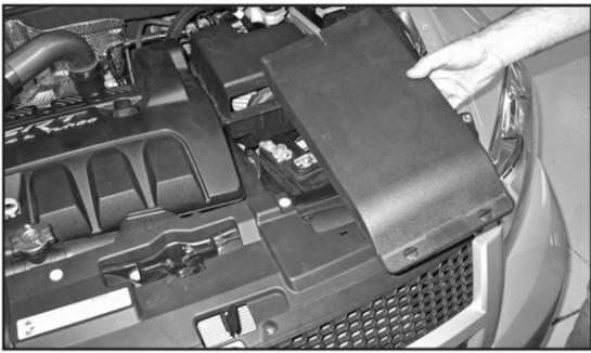
3. Remove the fresh air intake scoop from the vehicle.
