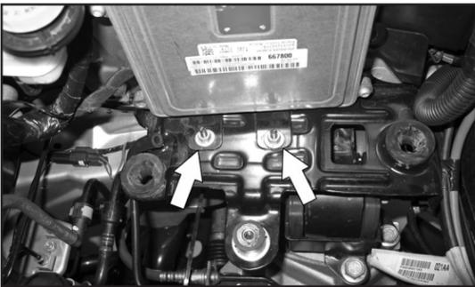
14. Remove the two ECU mounting nuts shown. **NOTE: These nuts will be reused in a later step.**
