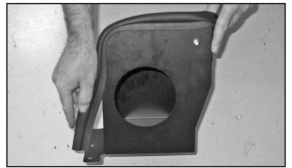
22. Install the provided edge trim onto the heat shield as shown. **NOTE: Some trimming of the edge trim will be necessary.**
