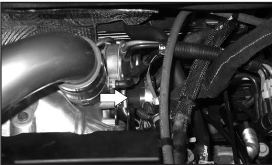
15. Install the provided silicone hose (08095) onto the turbo inlet and secure it with the provided hose clamp.
