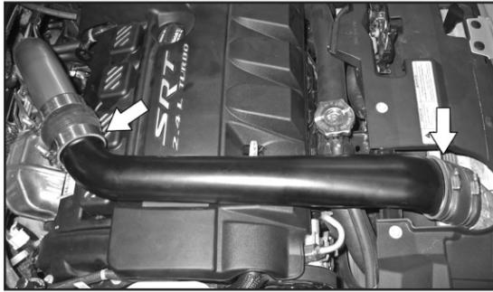
6. Loosen the two hose clamps that secure the intercooler transition tube. Then remove the intercooler transition tube.
