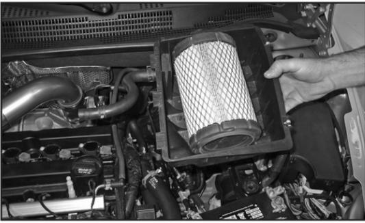
10. Lift up the air box to dislodge it from the mounting grommets. Then remove the air box from the vehicle.
