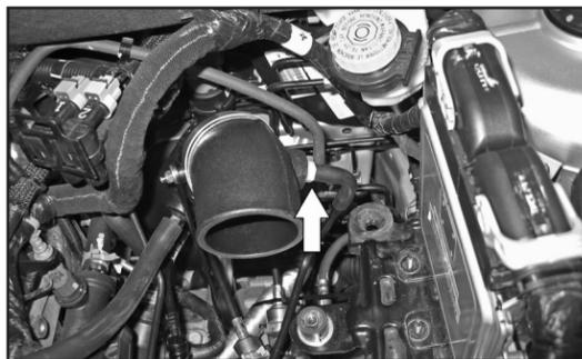
21. Attach the remaining vent hose to the 1/4NPT X 3/8" vent fitting installed in the K&N® intake tube.
