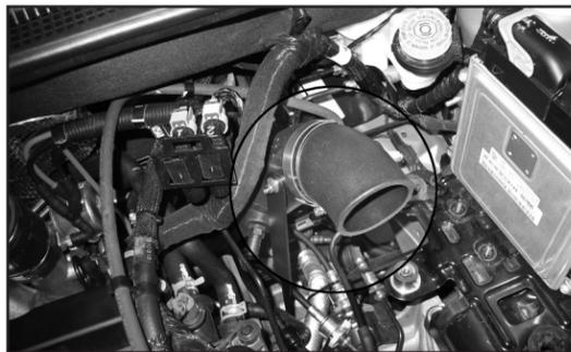
19. Install the K&N® intake tube into the silicone hose at the turbo inlet and align with the mounting bracket, then secure with the provided hose clamps.
