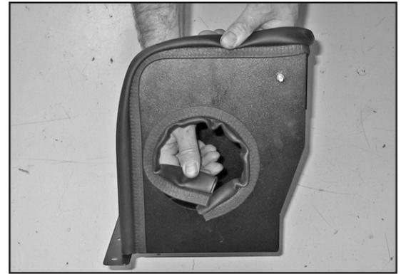
23. Install the provided edge trim into the hole of the heat shield as shown. **NOTE: Some trimming of the edge trim will be necessary.**
