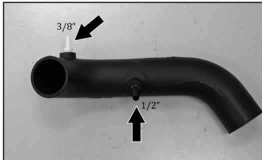
18. Install the two 1/4NPT fittings into the K&N® intake tube as shown. **NOTE: Plastic NPT fittings are easy to cross thread. Install the vent fitting "hand" tight, then turn it two complete turns with a wrench.**
