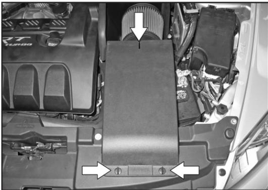
29. Install the fresh air intake duct onto the core support and heat shield, and then secure with the factory 1/4 turn clips and hardware provided.
