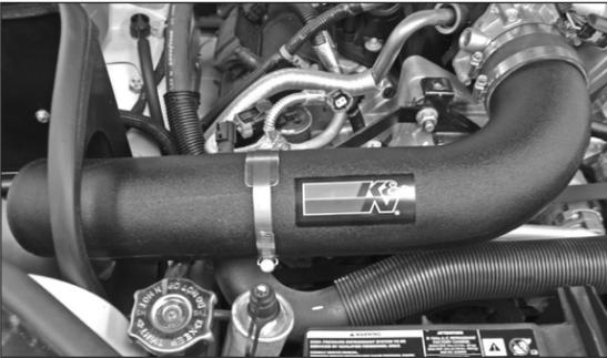
30. Install the intake tube into the silicone hose at the throttle body and onto the saddle clamp, then secure with the provided hose clamps.
