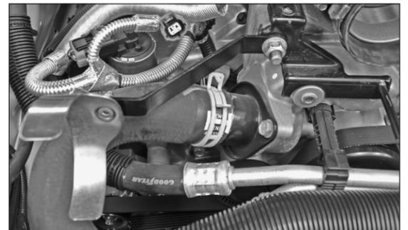
25. Install the tube mounting bracket assembly onto the plenum mount and secure with the factory nut removed in step #23.
