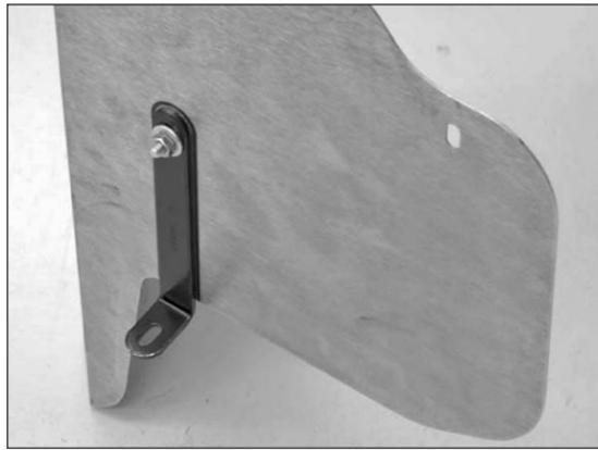
16. Install the large "L" bracket (26626) onto the heat shield as shown with the provided hardware.
