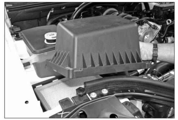
9. Unhook the air box lid retaining clamps and then remove air box lid and filter.
