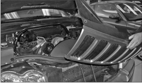
11. Remove the six grill retaining clips from the grill, then tilt the grill forward and lift to remove from the vehicle.
