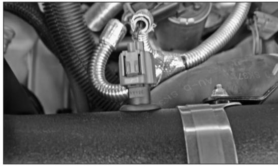
32. Reconnect the air temperature sensor electrical connection as shown.
