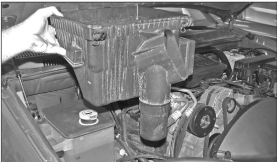
14. Lift the lower air box and remove it from the vehicle as shown.
