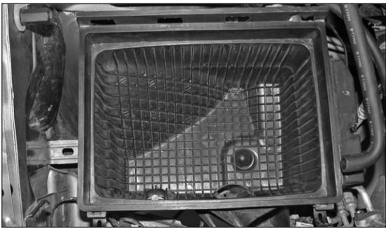
13. Remove the air box mounting bolt shown.
