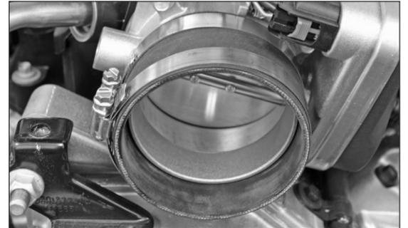
22. Install the silicone hose (08630) onto the throttle body and secure with the hose clamp provided.
