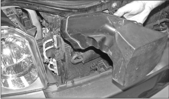
12. Pull the fresh air duct forward to disconnect it from the air box and then remove it from the vehicle.
