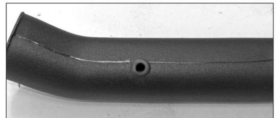
26. Install the provided grommet into the intake tube as shown.
