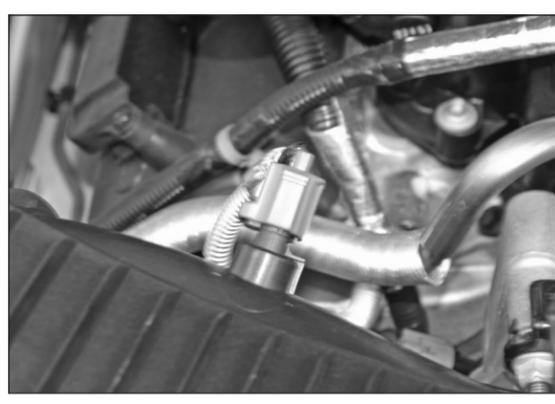
6. Disconnect the air temperature sensor electrical connection and then remove the intake plenum from the vehicle.
