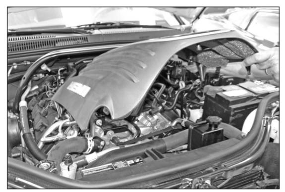
7. Remove the engine cover from the engine as shown.
