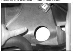
14. Feed the cold air hose down and through the hole in the under tray.
