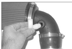
10. Screw the plastic elbow into the plastic intake pipe as shown.
