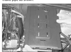
11. Remove the lid from the battery housing.
