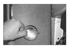
18. Locate the cold air hose through the hole in the base of the heat shield and secure in position using the 2 plastic ties supplied.
