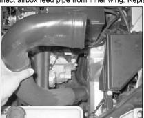
8. Carefully remove the original air box feed pipe from the vehicle.
