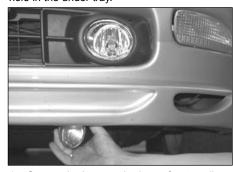
15. Secure the hose to the lower front spoiler screw hole using one of the plastic ties supplied.
