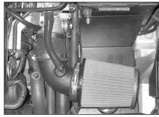
23. Carry out a final check of the alignment / fitment of the K&N induction system, ensuring that all clips etc are tight before starting the engine. Installation is now complete.
