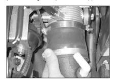
19. Fit the filtercharger assembly to the throttle housing and secure using the hose clip supplied.
