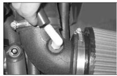
20. Fit the silicon breather hose from the throttle housing to the elbow on the plastic pipe.
