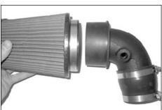
9. Assemble the filtercharger, rubber filter adaptor, plastic intake pipe and stepped silicone adaptor as shown using the hose clips supplied.
