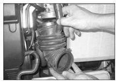
4. Unclip the intake hose from the throttle housing & carefully remove the pipe from the vehicle.
