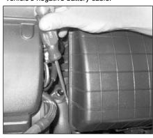
2. Unclip the intake hose from the air box lid.
