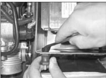
12. Fit the studded rubber mounting to the original hole in the battery housing using a flat washer and M6 nut supplied + refit battery cover.
