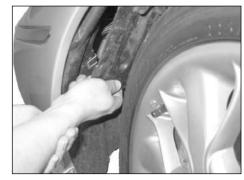
7. Remove the cover from the front left hand arch + disonnect airbox feed pipe from inner wing. Replace cover.
