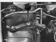
8. Refit the upper air box-mounting bracket & secure with the original screw.
