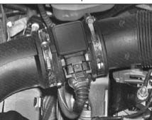
3. Unclip & remove the harness plug from the MAS (Mass Air Sensor).
