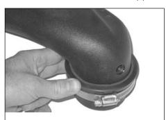
15. Fit the stepped rubber adaptor to the end of the new plastic intake pipe using a #60 hose clamp supplied.
