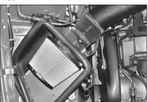
25.Fit the new Filtercharger to the intake pipe / filter adaptor, ensure the filter sits flush with the heat shield, fully tighten the #72 hose clamp supplied.
