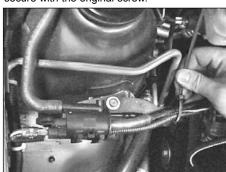
9. Secure the CFSV & any harnesses to the bracket using the plastic ties supplied.
