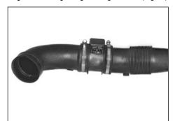
14. Remove the MAS from the 2 intake pipes.
