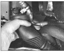
2. Remove the flexi intake pipe between the air box lid & intake scoop
