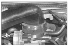
19. Attach the new intake pipe assembly to the throttle housing using the #60 hose clamp supplied.
