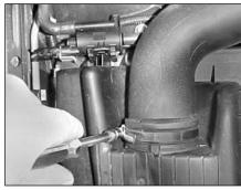
5. Unclip & remove the intake pipe from the
