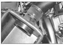
23. Fit the heat shield to the intake pipe assembly, ensure the rubber adaptor lip sits up against the shield.
