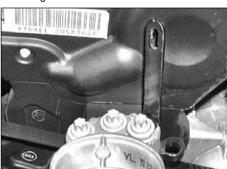
13. Secure the new mounting bracket to the engine mounting using the original bolt. (Fig.12)
