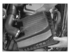
7. Slide the air box out of the lower mounting & carefully remove the complete air box from the vehicle
