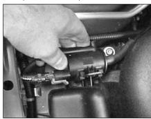
4. Unclip the CFSV (Carbon Filter Solenoid Valve) from the top of the air box lid.
