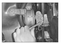
12. Remove the front bolt from the side engine mounting.
