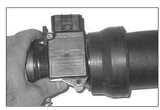
17. Fit the MAS to the other end of the new intake pipe using the stepped adaptor & #60 clamps supplied.
