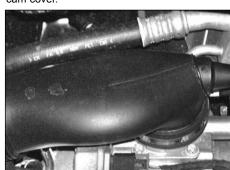
11. Unclip & remove the intake pipe assembly from the throttle housing. (Fig.10)
