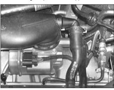
10. Remove the top plastic engine cover. Remove the engine breather hose from the cam cover.
