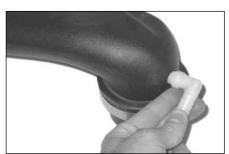
16. Screw the angled vent adaptor into the threaded hole on the side of the new intake
