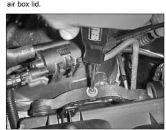
6. Remove the torx head screw securing the upper air box-mounting bracket.
