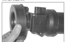
18. Fit the rubber filter adaptor onto the end of the MAS.
