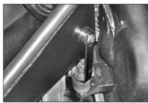
24. Attach the bracket to the mounting hole in the side of the heat shield using the nylon spacer, allen head bolt, nylock nut & washers supplied.
