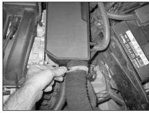
2. Unclip the rubber band securing the resonator box / intake hose.
