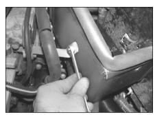
18. Secure the heat shield to the mounting bracket using a allen head bolt, nylock nut & washers supplied.
