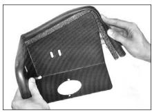
17. Clip the edge trim seal to the outside edge of the heat shield as shown (trim any excess seal).
