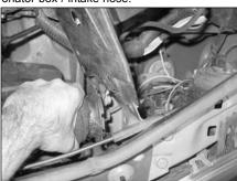
3. Unclip & remove the intake hose / scoop from the side air deflector.
