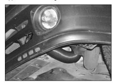
21. Feed the flexi cold air hose into the L/H lower grille, secure the hose to the grille using the plastic ties supplied. Secure the hose to the arch liner using a plastic tie supplied.
