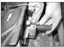
24. Fit the new 5/8"ID x 3"L silicone hose to the breather pipe located just below the throttle housing using a #8 hose clip supplied.
