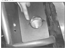
19. Pierce/drill two holes in the top of the flexi cold air hose to match the holes in the bottom of the heat shield. Attach the flexi hose to the hole in the bottom of the heat shield using 2 plastic ties supplied.
