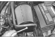
29. Set the height of the filtercharger on the slotted hole, then secure using a nylock nut & washer supplied.
