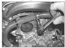
13. Secure the hose to the threaded hole on the side of the engine using the 'P' clip, allen head bolt & flat washer supplied.
