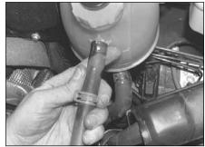
11. Carefully unclip & remove the coolant hose located between the coolant reservoir & thermostat housing (ensure that the cooling system is fully cold & depressurized before carrying out this operation).
