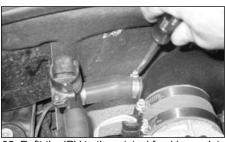
32. Refit the IRV to the original feed hose. Join the IRV / silicone hose to the new intake pipe using a #10 hose clip supplied.
