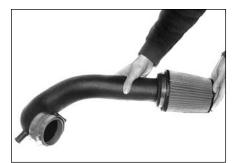
22. Assemble the new intake pipe using the silicone hose adaptor, rubber filter adaptor, filtercharger & hose clips supplied.
