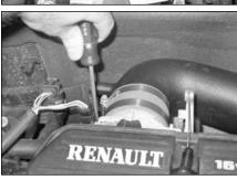
26. Fit the silicone adaptor hose / intake pipe to the throttle housing & secure using the #48 hose clip supplied.
