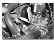
16. Fit the new mounting bracket to the engine lift bracket lower mounting hole using the original bolt.
