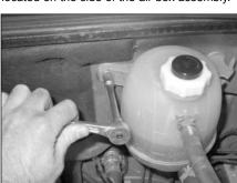
7. Remove the 2 nuts securing the coolant reservoir. Reposition the reservoir to allow sufficient clearance for carrying out instruction #9.
