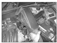
4. Remove the resonator box assembly from the vehicle. Unbolt & remove the intake hose support frame from the engine lift bracket.
