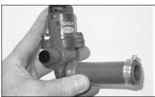
31. Fit the new 3/4"ID x 3"L silicone hose to the IRV using a #10 hose clip supplied.
