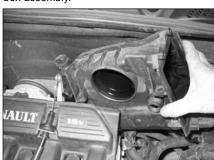
9. Pull the air box from the throttle housing & carefully maneuver the air box from the vehicle.
