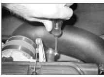
27. Secure the silicone breather hose using a #8 hose clip as shown.
