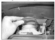
23. Remove the rubber 'O' ring seal from around the throttle housing.
