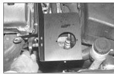
7. Attach the heat shield to the mounting bracket using the allen head bolts, nylock nuts & washers supplied (Fit two of the flat washers between the bracket & shield). Align the heat shield to finish as low & level as possible, ensuring sufficient clearance between the bonnet...
