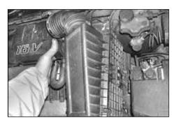
4. Unclip the feed pipe from the base of the air box, carefully lift the complete air box assembly out of its lower mountings & remove the assembly from the vehicle.
