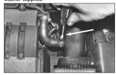
14. Fit the new breather hose to the intake pipe & engine breather pipe on the cam cover, secure using the small hose clips supplied.
