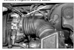
2. Unclip & remove the intake hose from the throttle housing.
