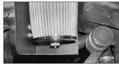
12. Fit the studded lid of the filtercharger to the slotted hole in the front of the heat shield using the plastic spacer.
