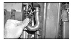
3. Unclip & remove the engine breather hose from the side of the cam cover.
