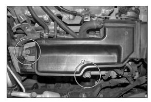
5. Remove the two bolts that secure resonator assembly to the motor.
