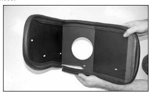
10. Apply the edge trim to the heat shield as shown above. Trim excess as needed.
