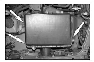
7. Loosen the three bolts that secure the air cleaner assembly to the inner fender.
