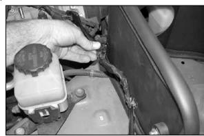
18. Insert mass air wire retaining clips into holes provided in heat shield.
