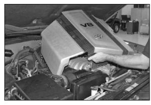
2. Remove the two bolts and two nuts that secure the engine cover, then remove the engine cover.
