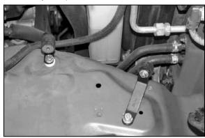
15. Install bracket (070782) with rubber mounted stud onto vehicle with provided hardware.
