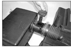
19. Remove two screws securing mass air sensor to stock intake tube, then remove mass air sensor from tube.
