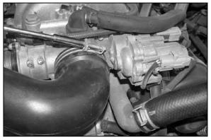
6. Loosen the hose clamp at the throttle body as shown.
