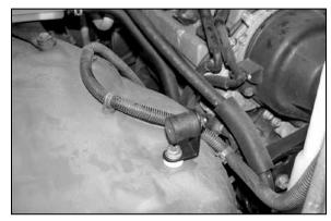
14. Install small "L" bracket with 3/4" rubber mounted stud to the inner fender as shown with provided nylon spacer and hardware.
