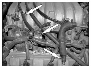
9. Remove the EVAP canister vent hose, the crank case vent hose and the fuel pressure regulator vent hose.
