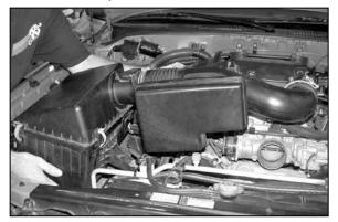
8. Remove the intake tube from the throttle body, then remove the complete air intake assembly. NOTE: K&N Engineering, Inc., recommends that customers do not discard factory air intake.
