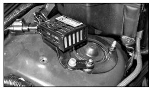
15. Install the new K&N<sup>®</sup> bracket onto relay and then onto strut mount as shown. Tighten all hardware completely.
