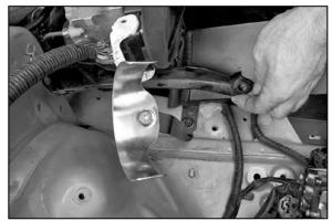
20a. On 2002 and later models, lift up on the ABS bracket and mount the heat shield and saddle bracket assembly onto the vehicle with the provided 8mm button head bolt as shown.
