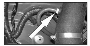
31. Connect the other end of the silicone hose onto the K&N $^{\circ}$  intake tube as shown.
