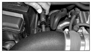
32. Reconnect the crank case vent as shown.
