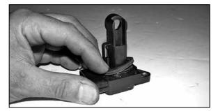
23. Install the provided gasket onto the mass air sensor with the sticky side towards the mass air.
