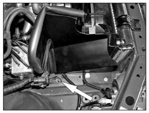
18. Install heat shield onto the vehicle and fasten to the vehicle with the provided 6mm bolt as shown. NOTE: The heat shield needs to be mounted under ABS pump bracket.
