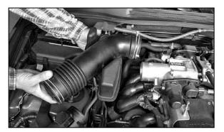
7. Remove the intake tube as shown.
