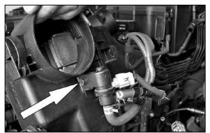
10. Lift air box up to access the 10mm bolt that retains the evap Solenoid to the air box then remove bolt.
