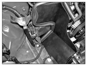
20. On 01 models, mount the heat shield and saddle bracket assembly onto the vehicle with the provided 8mm button head bolt as shown.
