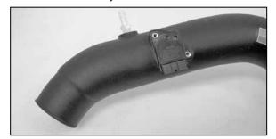
24. Install the mass air onto the new K&N<sup>®</sup> intake tube with the provided hardware as shown.
