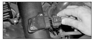
35. Reconnect the mass air electrical sensor as shown.
