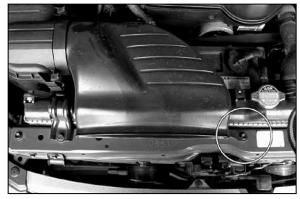
8. Loosen and remove the 10mm bolt that retains the fresh air intake to the vehicle then remove from the vehicle.
