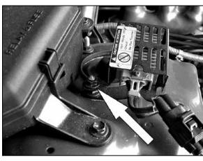
13. Loosen the 12mm nut. **NOTE: Do not remove nut.**
