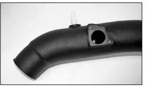
21. Install the vent fitting onto the new  $K\&N^{\circledast}$  intake tube as shown.
