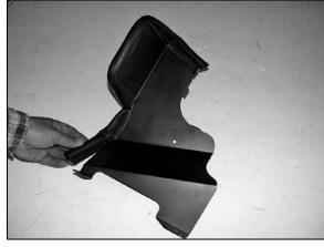
16. Install edge trim onto the heat shield as shown. Trim if needed.
