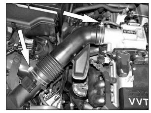
6. Loosen the 2 hose clamps that secure the intake tube to the air box and the throttle body.
