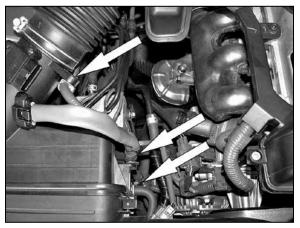
4. Remove the 3 clips that retain the electrical harness onto the factory air box.
