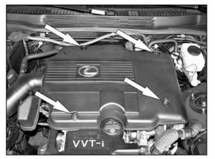
2. Loosen and remove the 4 nuts that retain the engine cover to engine then remove the engine cover.
