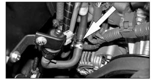
30. Connect the provided hose onto the evap solenoid as shown.
