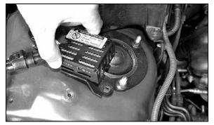
14. Loosen and remove the 12mm nut then lift and rotate relay box clockwise as shown.
