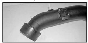
26. Install the filter adapter onto the  $K\&N^{\circledast}$  intake tube as shown.
