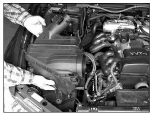
12. Remove the complete air box from vehicle.
