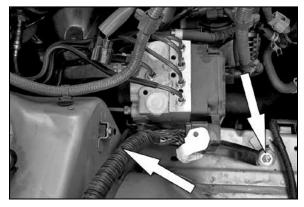
17a. On 2002 and later models, loosen and remove the 2 bolts and one nut that retains the ABS pump to the vehicle.
