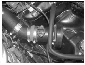
26. Install the mass air assembly onto the K&N<sup>®</sup> intake tube and secure with the provided hose clamps as shown.
