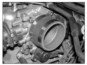
14. Install silicone hose (08186) onto the throttle body with the provided hose clamps.
