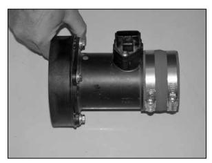
25. Install the silicone hose (08434) onto the mass air sensor with the provided hose clamps as shown.
