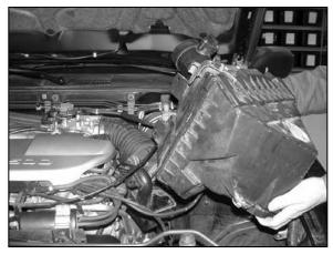
6. Remove the airbox assembly from the vehicle.
