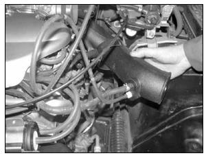
16. Install the vacuum lines removed in step #3 onto the K&N® intake tube as shown.
