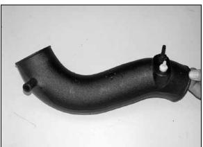
15. Install the provided NPT fittings onto the K&N<sup>®</sup> intake tube as shown.
