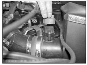
29. Reconnect the mass air sensor electrical connections.
