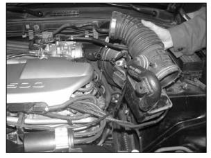
10. Remove the intake tube assembly from the vehicle.
