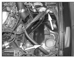
22. Install the K&N<sup>®</sup> heatshield into the vehicle using the provided hardware.
