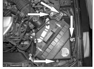
4. Loosen the intake tube hose clamp at the mass air sensor, then remove the two air box mounting nuts and the two air box mounting bolts.
