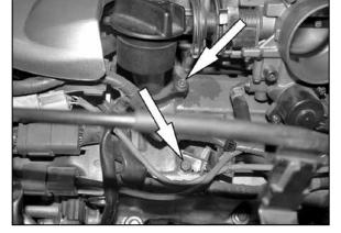
11. Remove the oil fill retaining bolt and the wire harness clip retaining bolts shown.
