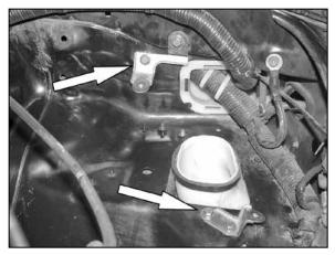
7. Remove the four bolts securing the two air box mounts and remove the mounts.
