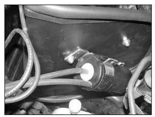
22a. On vehicles equipped with the SCV vacuum tank using the hardware provided, bolt the tank to the lower "L" bracket bolt and through the hole in the heatshield as shown.
