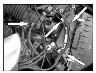
3. Unclip the vacuum lines from the air filter box, then disconnect the vacuum lines from the airbox and intake tube.
