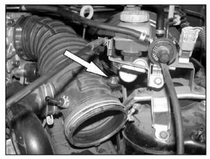
9. Loosen the intake tube hose clamp at the throttle body and remove the intake tube mounting bolt shown.
