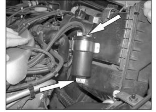
5. On vehicles equipped with SCV vacuum tank, lift the air box and twist to gain access to the SCV vacuum tank retaining bolts and remove, set SCV vacuum tank aside.
