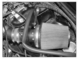
27. Install the K&N<sup>®</sup> filter charger onto the mass air adapter and secure with the provided hose clamp. NOTE: Drycharger® air filter wrap; part # RF-1037DK is available to purchase separately. To learn more about Drycharger® filter wraps or look up color availability please visit http:// www.knfilters.com®.
