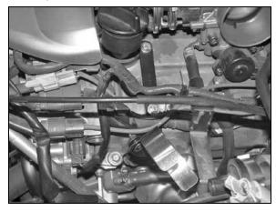
13. Install the saddle bracket assembly onto the valve cover using the hardware provided, threaded into the holes accessed in step #11.
