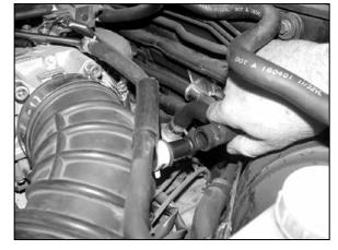
8. Loosen the spring clamp on the crank case vent hose, then disconnect the crank case vent hose from the intake tube.
