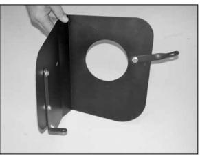
19. Install the twist bracket (07945) onto the heatshield with the provided hardware as shown.
