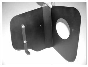
18. Install "L" bracket (070902) onto the heatshield with the provided hardware as shown.
