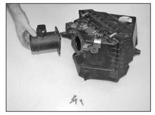
23. Remove the four bolts that secure the mass air sensor to the air box and remove the mass air sensor from the air box.
