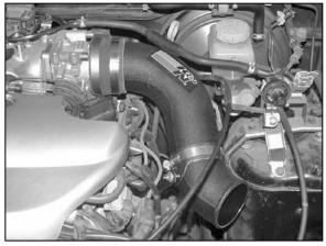
17. Install the K&N<sup>®</sup> intake tube onto the throttle body and saddle bracket, secure with the provided hose clamps.
