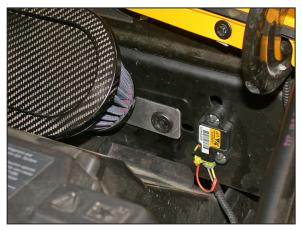
12. Snap the filter-mounting bracket onto the filter as shown and secure with the provided hardware.
