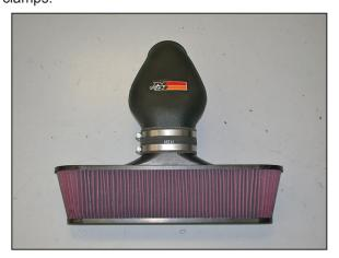
8. Install the K&N® intake tube onto the air filter as shown and secure with the provided hose clamp.
