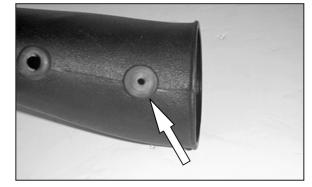
23. On models equipped with a fuel pressure regulator vacuum line, insert the 3/16" ID grommet into the hole drilled in the previous step.
