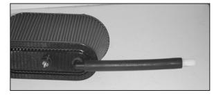
12. Detach the wiring harness retaining clip from the lower radiator cover.
