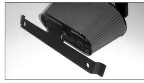
29. Attach the angled bracket to the rubber mounted stud using the provided hardware. Note: Do not tighten completely at this time.
