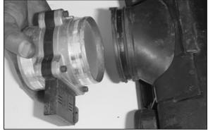
16. Remove the mass air sensor from the airbox.
