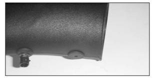
24. Insert the air temperature sensor into the  $1/2\ensuremath{"}$  ID grommet.
