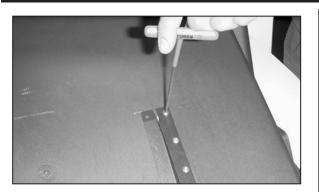
48. Secure the bracket to the lower radiator cover with the hardware provided.
