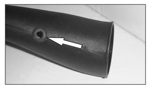
21. Insert the 1/2" ID grommet into the hole in the K&N $^{\odot}$  intake tube.
