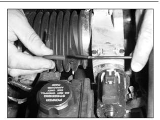
5. On models equipped with a fuel pressure regulator vacuum line, disconnect the vent hose
