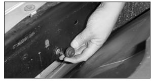
17. Remove the two grommets from the airbox mounting points.
