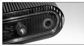
20. Install the 5/8" ID grommet and the rubber mounted stud into the top plate of the Air filter element.
