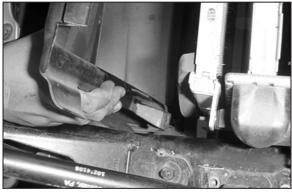
42. Pull firmly to release the radiator cover from it's retaining clips.
