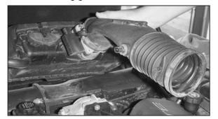
11. Detach the intake hose from the throttle body and remove the entire air intake assembly. **NOTE: K&N Engineering, Inc., recommends that customers do not discard factory air intake.**
