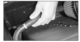
59. Attach the air injection hose to the hose mender.
