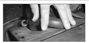
7. Disconnect the air injection vent hose.
