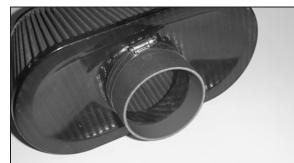
18. Attach the 3.5" ID silicone hose (08630) onto the flange of the Air filter element.
