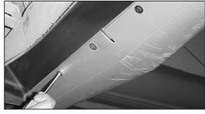
39. Loosen and remove the five bolts that mount the lower radiator cover to the bumper cover on the underside of the car.
