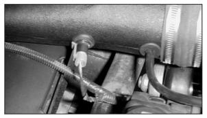
64. Reconnect the air temperature sensor electrical connection.
