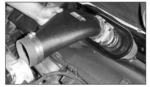
32. Install the K&N® intake assembly.
