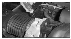
9. Loosen the hose clamp on the intake hose at the throttle body.
