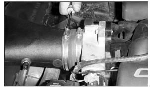
60. Attach the silicone hose to the throttle body and tighten the hose clamps.
