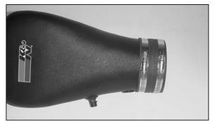
27. Install the 4" ID silicone hose onto the K&N $^{\mbox{\scriptsize \$}}$  intake tube.
