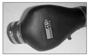
28. Install a 3.5" ID silicone hose (08630) onto the K&N<sup>®</sup> intake tube.
