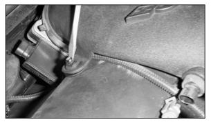
8. Release the push clips that retain the stock intake tube to the upper radiator cover.
