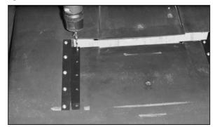
50. Drill out the five inner holes of each bracket.
