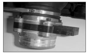
15. Remove the mass air sensor retaining clamp.
