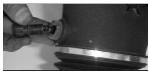
14. Remove the air temperature sensor from the stock intake tube.
