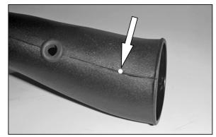
22. On models equipped with a fuel pressure regulator vacuum line, drill out the drill point in the K&N<sup>®</sup> intake tube using a 3/4° drill bit.
