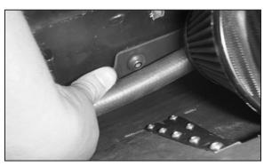
57. Install the angled bracket onto the original airbox mounting points.
