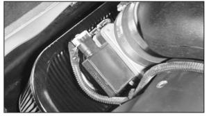
63. Reconnect the mass air sensor electrical connection.
