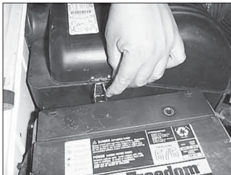
4. Release the over center clips and remove the airbox top.
