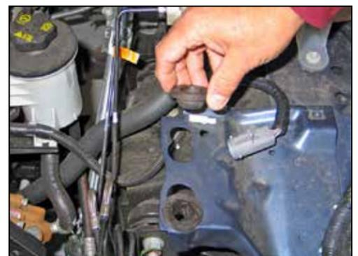
6. Remove the two air box mounting grommets from the bracket as shown.
