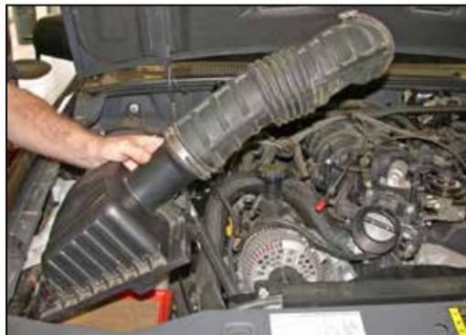
6. Loosen the hose clamp which secures the intake tube to the throttle body, release the two clam shell clamps which secure the upper airbox lid and then remove the airbox lid and intake tube from the vehicle.
