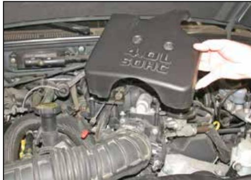
4. Remove the engine cover from the engine.
