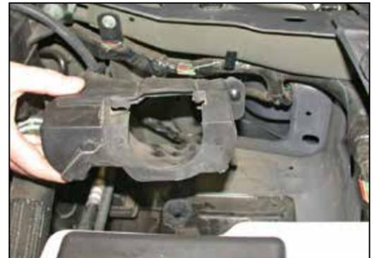
8. Pull firmly on the air duct to dislodge it from core support and remove from the vehicle.
