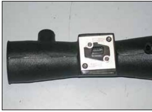
15. Secure the mass air assembly onto K&N® intake tube using the hardware provided as shown.
