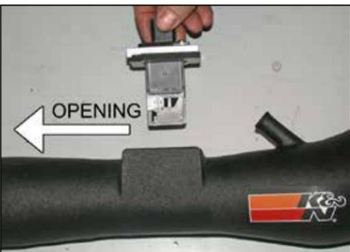
14. Install the mass air sensor assembly into the K&N® intake tube as shown.
