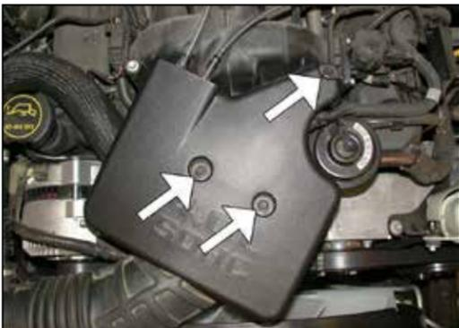
3. Remove the three- engine cover mounting bolts shown.
