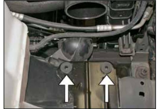
21. Install the two provided threaded inserts into the lower airbox mounting plate as shown.
