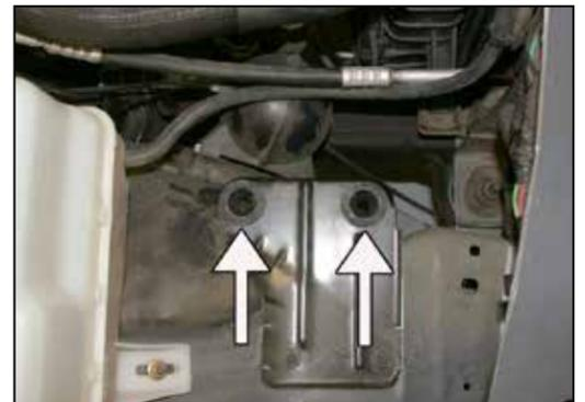
9. Remove the two-airbox mounting grommets from the mounting plate shown.
