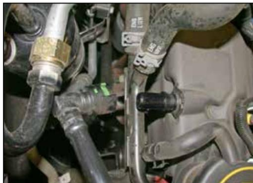
5. Depress the green locking tab on the crankcase vent hose attached to the valve cover of the engine and then disconnect the vent hose from the valve cover as shown.
