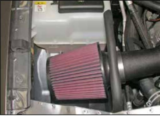
25. Install the air filter and secure with hose clamp provided.
