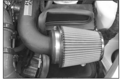
19. Install the air filter onto the intake tube as shown.
