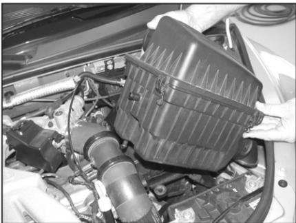
3. Lift firmly up on the airbox to remove from vehicle, then disconnect the crankcase vent from the airbox.
