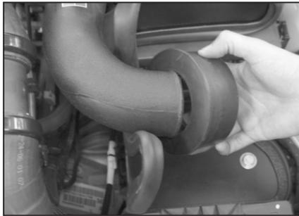
18. Install the air filter adaptor onto the intake tube as shown.
