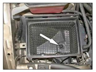
8. Remove the airbox mounting bolt shown.
