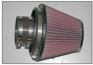
28. Install the silicone (08630) onto the air filter assembly and secure with the provided hose clamp.
