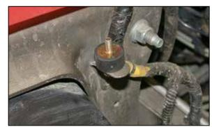
21. Install the 6mm male/male rubber mounted stud onto the upper airbox mount as shown.
