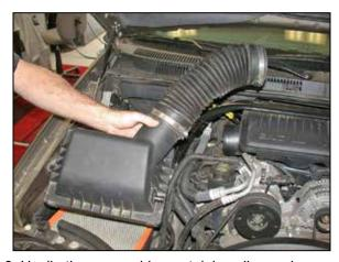
3. Unclip the upper airbox retaining clips and remove the upper airbox and intake tube assembly as shown.
