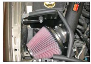
29. Install the air filter assembly onto the K&N® intake tube as shown and secure with the povided hose clamp.
