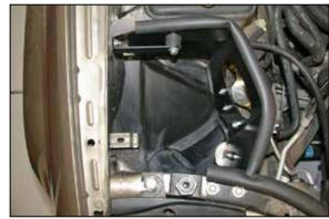
22. Install the heat shield assembly into the vehicle and secure it to the mounting locations with the provided hardware.
