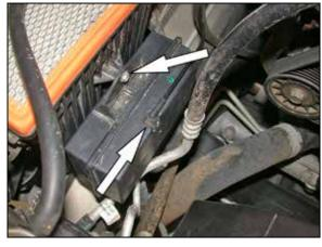
4. Disconnect the vacuum canister hose shown.
