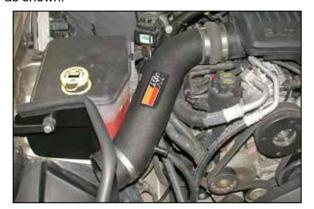
25. Install the K&N® intake tube into the silicone hose at the throttle body and onto the saddle clamp, then secure with the provided hose clamps as shown.
