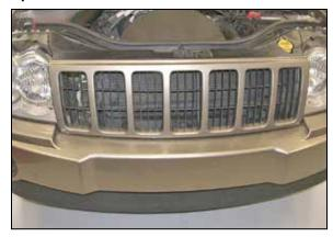
30. Reinstall the grill assembly with the factory retaining clips removed in step #5
