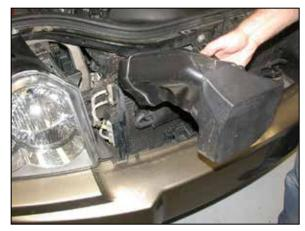
7. Pull the fresh air duct forward to disconnect it from the airbox and then remove it from the vehicle.
