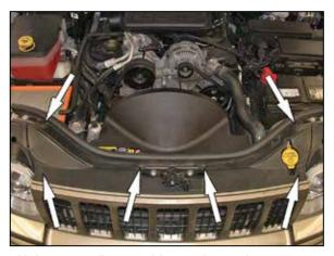
5. Using a small screwdriver, release the center holding pins in the six grill retaining clips shown.
