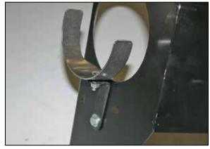
12. Install the saddle bracket assembly onto the heat shield with the provided hardware as shown.
