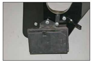
18. Using the provided spacer, install the vacuum reservoir onto the heat shield as shown.
