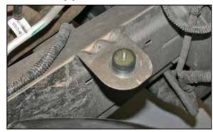
20. Using the two fender washers and one rubber washer, install the 6mm male/female rubber mounted stud onto the lower airbox mount as shown.
