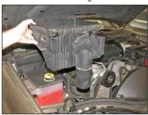
9. Lift the lower airbox and remove it from the vehicle as shown.
