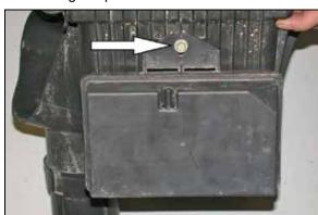
17. Remove the bolt which secures the vacuum reservoir to the airbox and then remove the reservoir from the airbox.
