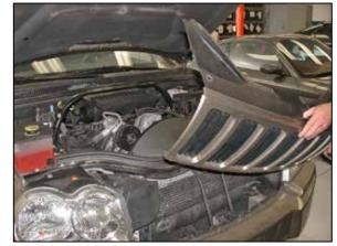
6. Remove the six grill retaining clips from the grill, then tilt the grill forward and lift to remove from the
