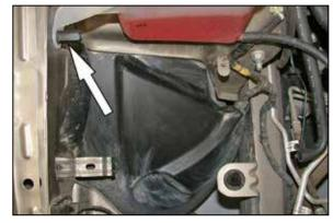
19. Remove the coolant reservoir-retaining nut and airbox mounting grommet shown.
