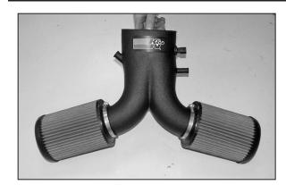
10. Install the air filter onto the K&N® intake tube.
