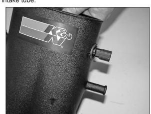
9. Install the air temp sensor into the K&N<sup>®</sup> intake tube.
