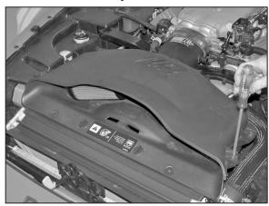
12. Reinstall upper airbox coer removed in step #4 and tighten six mounting screws.
