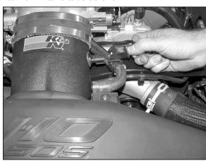
15. Reconnect air temp sensor electrical connection.
