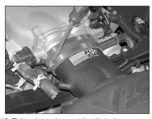
13. Tighten hose clamps at throttle body.
