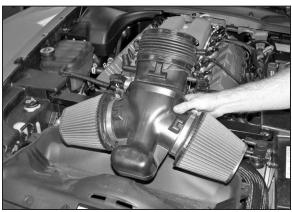
5. Loosen intake tube hose clamp at throttle body, and remove wing nut under tube. Then remove complete intake assembly.
