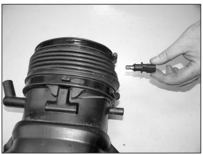
8. Remove the air temp sensor from the stock intake tube.
