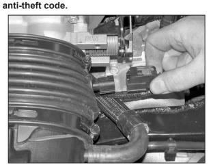
2. Disconnect air temp sensor electrical connection.
