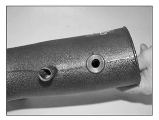
7. Install the provided rubber grommet into  $K\&N^{\scriptsize \circledcirc}$  intake tube.
