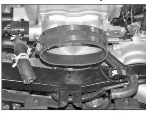
6. Install silicone hose (08540) onto throttle body with hose clamps provided.
