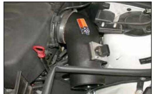
21. Attach the K&N® intake tube to the plenum with the provided hose clamp.
