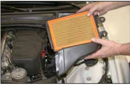
7. Remove the lower air box assembly as shown.
