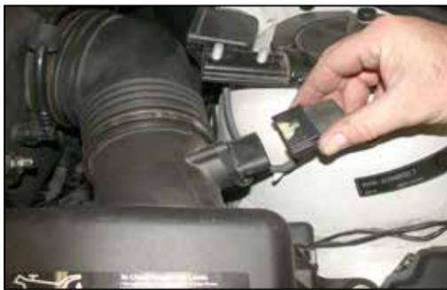
3. Squeeze the two locking tabs together, then remove the mass air electrical connection as shown.
