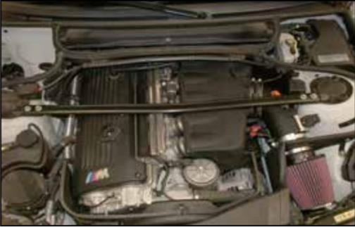
26. Re-install the strut tower brace that was removed in step 2.
