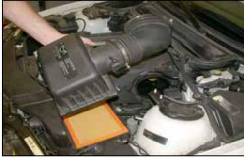
4. Loosen the hose clamp at the intake plenum and release the two clips that secure the air box lid to the vehicle. Remove the upper air box and intake tube as shown.
