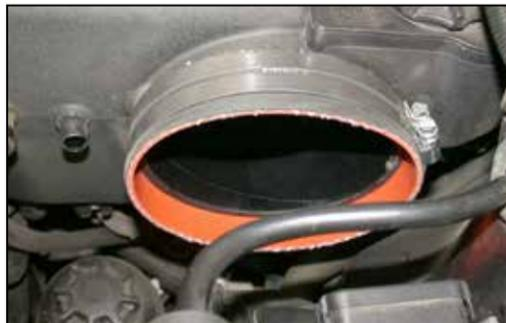
15. Install the silicone hose (08612) onto the intake plenum as shown using the provided hose clamps.
