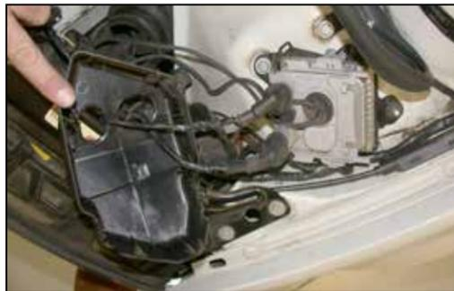
14. Re-install the head light module with the original hardware that was removed in step 5.
