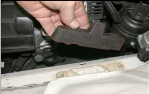
8. Lift up on lower air box mount and then remove from vehicle.
