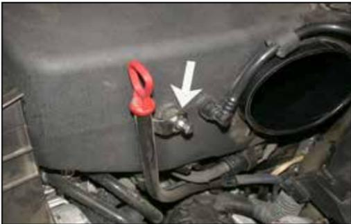
9. Remove the nut that secures the dip stick to the intake plenum.
