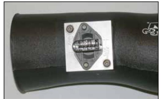
20. Secure the mass air sensor assembly into the K&N® intake tube with the provided hardware as shown.
