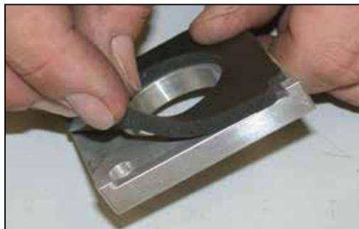
17. Install the provided gasket onto the mass air adapter as shown, sticky side down.
