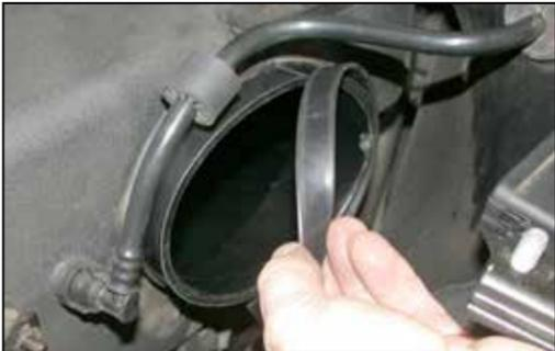
10. Remove the intake o-ring from the plenum as shown.
