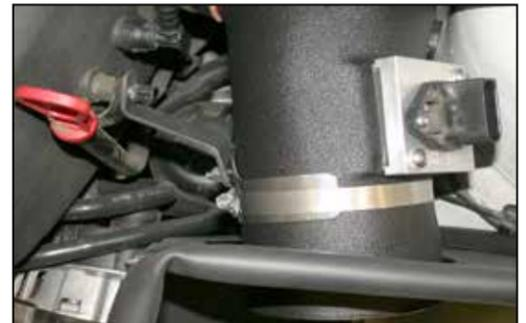
23. Attach the saddle bracket assembly to the intake plenum with the nut removed in step 9, then attach the saddle bracket to the intake tube with the provided hose clamp.
