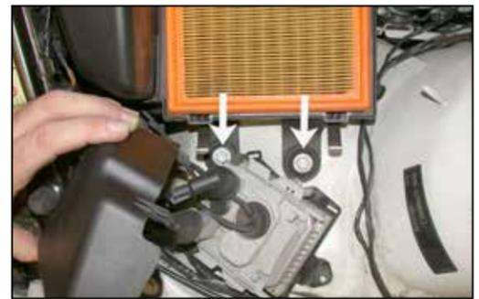
5. Remove the cover to the head light module to gain access to the air box bolts and module nut. Remove the bolts and nut.
