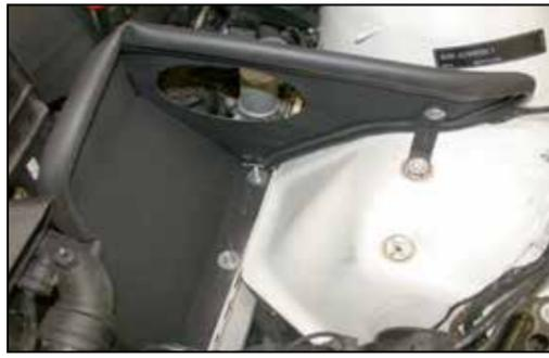
13. Secure the heat shield to the vehicle with the provided hardware. Secure bracket (010090) to the heat shield and inner fender.
