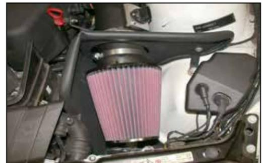
24. Install the K&N® air filter onto the K&N® intake tube and secure with the provided hose clamp.
