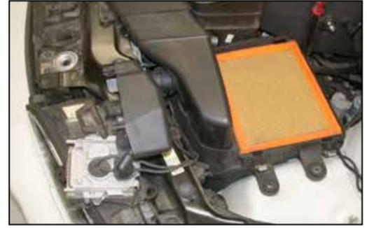
6. Lift the head light module and place out of the way on the core support to gain access to the lower air box for removal.
