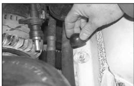
12. Unthread and remove the air box locating bumper.
