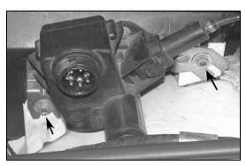
3. Remove the two speed control mounting nuts, then lift and place the speed control unit to the
