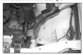
11. Remove the fresh air duct from the vehicle as shown.
