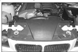
23. Re-install the radiator cover removed in step #9 and secure with the existing hardware.
