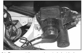
21. Reconnect the speed control electrical connection and twist the locking ring clockwise to lock in position.
