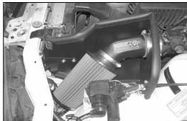
22. Install the K&N $^{\!\scriptscriptstyle \otimes}$  air filter and secure with the provided hose clamp.
