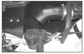
20. Re-install the speed control removed in step #3 to the mounting brackets with the provided hardware as shown.
