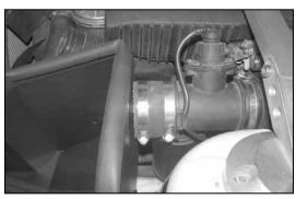
17. Install silicone hose (08690) onto the mass air sensor as shown with the provided hose clamps.
