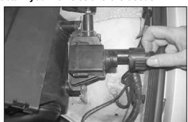
2. Twist the locking ring on the speed control electrical connection counter clockwise, then separate the wire harness connection from the speed control.
