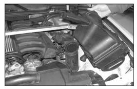
7. Remove the air box from the vehicle as shown. NOTE: K&N Engineering, Inc., recommends that customers do not discard factory air intake.
