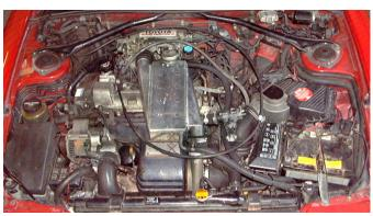
1. Unclip and remove the electrical harness plug from the AFM (Air flow meter)
