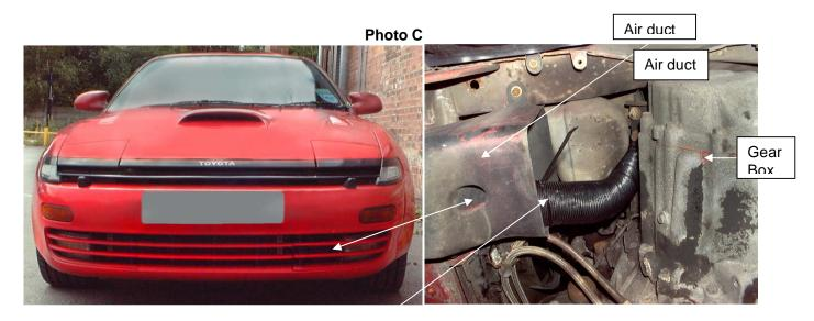
Taking all necessary safety precautions as per manufacturers instructions, raise the front of the car. 1. Unscrew and remove the lefthand undertray. Feed the flexi cold air hose up between the gearbox to the top of the engine bay, next to the battery. Feed the other end of the flexi cold air hose into the large plastic duct. Pierce/drill a 3mm hole in the duct and secure the hose to it with along plastic tie supplied. Refit the undertray.
