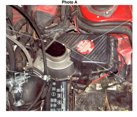
3. Unclip and remove the air box lid assembly.
