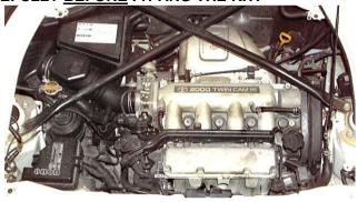
**1.** Release the hose clip and securing screw on the resonator box and remove from the intake hose.
