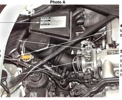
**4.** Remove the air temp sensor from the air box lid.
