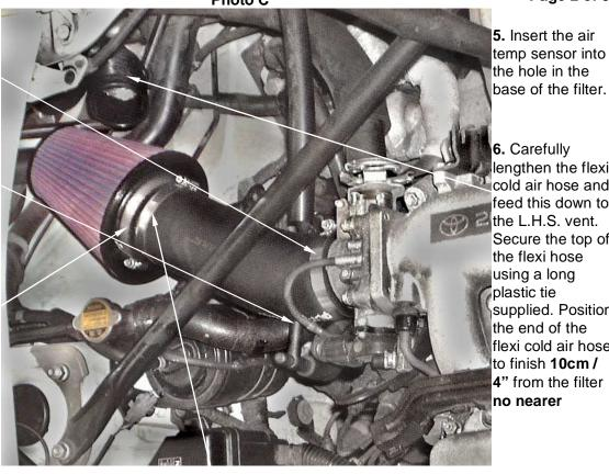
4. Fit the filter assembly in the intake hose, rotate the filter so the K&N logo is straight then tighten the #48 hose clip supplied.
