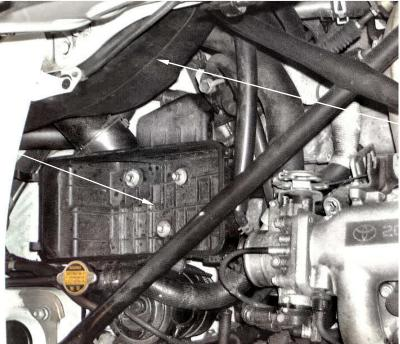
**2.** Remove the 3 bolts securing the air pick up box and remove from the car.
